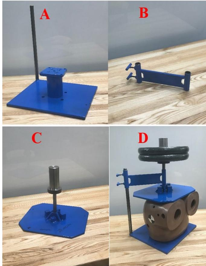
Figure 5: Test Stand Components: (A) Base Plate with Pedestal, (B) Support Arm, (C) Top Plate with Weight Mount, and (D) Complete Assembly with 75 lbs of Load
