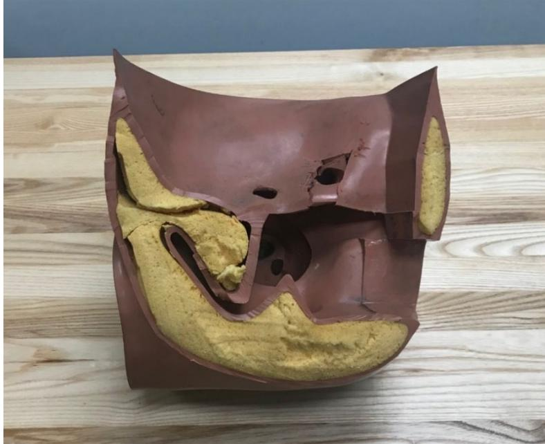
Figure 1: Pelvis Foam and Rubber Shell Cross Section
