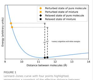
Lennard-Jones curve with four points highlighted, representing a snapshot of the effective distance between neighbors in both the relaxed and perturbed states of a mixture and a pure molecule.
