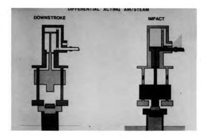
B9. The cycle is completed at the end of the up stroke when gas pressure is again applied in both the upper and lower chambers. The purpose of the double acting concept is to shorten the stroke and speed up the operation while maintaining about the same ram impact velocity. Typically, double acting hammers operate at about twice the speed of single acting hammers. As mentioned above, the differential acting hammer has been described. There are,
