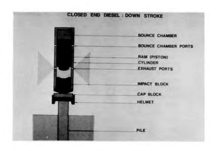
B32. Again when the ram passes the exhaust ports the gas in the combustion chamber is compressed.
