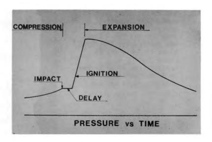
B29. Actually, the pressure will have a high frequency fluctuation which is induced by ignition. However, this phenomenon cannot be realistically modeled and it has no significant effect on the pile dynamic performance.
