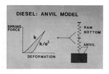
coefficient of restitution, e. The model below the impact block is identical with that used for the air/steam hammer.
