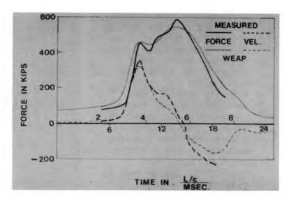
C38. The WEAP program is the first wave equation program to be extensively and systematically tested against field measurements of force and velocity. This testing activity has produced important changes in the program and a more correct model of driving systems. It has also shown again that correct input information must be available if meaningful results are to be obtained. In many cases the stateof-the-art makes the determination of input
