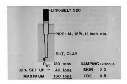
C26. A WEAP analysis with relatively high viscous damping factors of 2.0 and 0.8 for skin and toe, respectively, shows that the driving resistance would be 221 blows per foot at 120 tons resistance. It would be infinite, that is there would be no set, at the set up capacity of 160 tons. The conclusion is that the hammer/pile system would be insufficient if the pile had to be driven after a waiting period.
