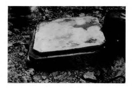
B43. The capblock is modeled as a spring with a steeper unloading portion to represent the coefficient of restitution.
