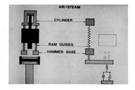
B14. The wave equation program begins by giving the ram element (or elements) the rated impact velocity. As impact occurs all segments of the wave equation model obtain a velocity and, therefore, move downward. The portions of the assembly segments are also continuously computed in their free fall. The motion of the pile segments causes the soil resistance forces to be activated. Once the pile has rebounded and all soil springs are
