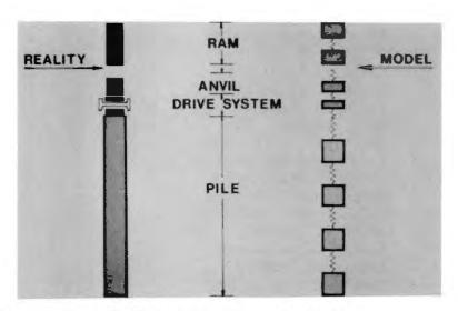
mass and spring characteristics can be calculated from the physical characteristics of the pile and the driving system.
