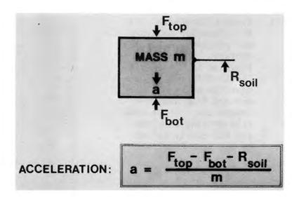
Al4. Having determined the acceleration of the element, its velocity and displacement can be determined by integration. For this integration a small time increment is used during which the acceleration is assumed constant. The results of the integration becomes more acourate as the time increment is made shorter. Of course, as the time increment is made shorter the
