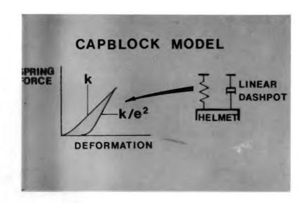
B44. The helmet is that steel element which contains the capblock on top and holds the pile in alignment with the appropriate recess in the bottom. It is modeled as a mass together with the mass of the capblock, strikerplates and pile adaptors, if present. If steel or timber piles are being driven the helmet fits directly on top of the pile.
