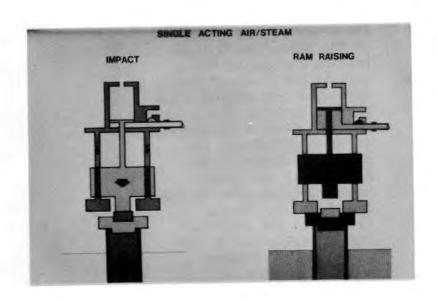
B6. In this slide a typical single acting air/steam hammer is shown. This particular machine has a 6,000 pound ram, a stroke of about three feet, and an operating speed of about 60 blows per minute.
