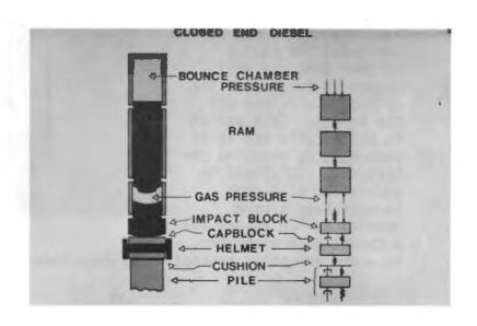
B38. Some hammers introduce the fuel in an atomized state. Thus, ignition occurs shortly after injection in a manner similar to the conventional diesel engine. Burning then takes place over a longer time depending on the rate of fuel injection.
