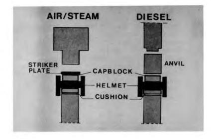
842. Capblocks formerly consisted of hardwood or cable coils. Increasingly artificial composite materials are used. These newer materials have the advantage of offering more uniform and reproducible mechanical properties.
