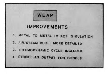
A27. models the total system will provide the best possible means of evaluating pile driving short of going to the field. In many cases it is impossible to provide the proper soil constants or to anticipate hammer performance. In such cases it is unrealistic to expect that the wave equation will predict the actual field performance. These problems can best be solved by field measurements using
