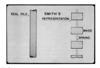
Al3. The forces acting on a typical pile element are those due to the strain at its top and bottom and to the soil resistance. Thus, from Newton's Second Law, the elements' acceleration at a particular time is equal to the sum of Ftop Fbottom, and Rsoil, divided by the mass of the element.
