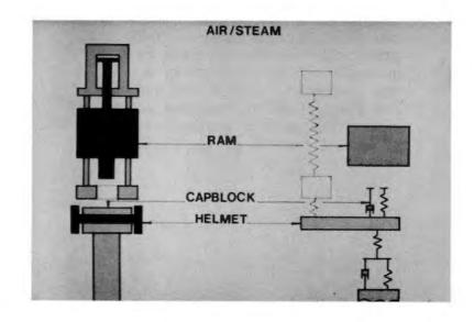
13b. The hammer assembly is also modeled by a series of masses and springs with the bottom spring at the interface of the assembly and the helmet also a compression -only spring. For the majority of currently available hammers, two masses are required; one representing the cylinder and the other, the hammer base. The connecting spring gets its flexibility primarily from the hammer columns.
