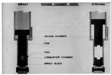
B41. So far only hammer models have been discussed. Now the next elements down in the driving system, the capblock, helmet, cushion model will be described. The capblock is that portion of the driving system which receives the impact force from the ram in the case of air/ steam hammers or from the impact block from diesel hammers.
