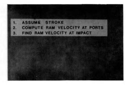
B26. As the ram moves down the combustion chamber pressure is calculated from the gas law. When the ram reaches the impact block the velocity is known and the wave analysis can be performed in a fashion similar to that described earlier.
