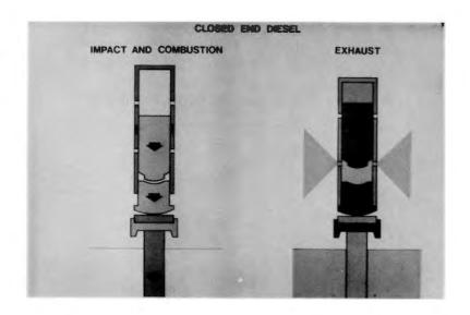
B35. As the ram continues on up fresh air is drawn into the combustion chamber and scavenging occurs. If the upward velocity of the ram is too great the bounce chamber pressure will become so large that the cylinder is lifted off the helmet. This action is undesirable and it is prevented by reducing the throttle. It should be understood that some hammers have a more complex system associated with the bounce chamber.
