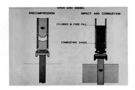
B18. As a result of the combined effect of the combustion chamber pressure and the pile rebound, the ram moves upward allowing an expansion of the combustion products. When it passes the exhaust ports the excess pressure is blown off.
