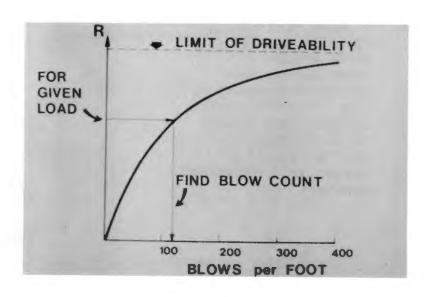
A10. Now consider the causes for problems with the dynamic formulas. First, the derivation is not based on a realistic treatment of the driving system nor does it recognize the variability of equipment performance. Typical driving systems can include many elements in addition to the ram such as helmet. capblock, cushion, and
