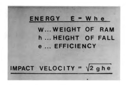
The mathematical model used in the WEAP program is more detailed than that which has been used previously. The ram can be represented by a series of masses and springs. The spring shown connecting the bottom ram element and the helmet is capable of carrying compression only. For currently available air/ steam hammers the rams are so stocky that they can be represented by a single mass element. The details of the modeling of the helmet-capblock assembly will be discussed later.
