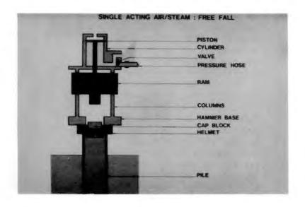
consisting of the hammer base, columns, and cylinder are all resting on the helmet (and, hence, on the pile top).
