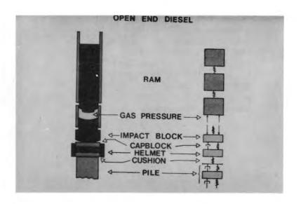
B23. The steel to steel impact of the ram on the impact block represents a particular problem and one which must be handled carefully. The research conducted during the development of the WEAP program leads to the use of an impact block spring which represents simply the combined stiffness of the last ram segment and the anvil. The spring is modeled with non-linear properties as are the springs of all cushion materials. The change of slope is identified by a
