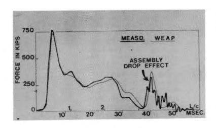
C33. The second test case was taken from a special test program on a DELMAG D-30 hammer. These tests were performed by Goble & Associates in 1971, for the Foundation Equipment Company of Newcomerstown, Ohio. In addition to force and velocity at the pile top the combustion chamber pressure was also measured.
