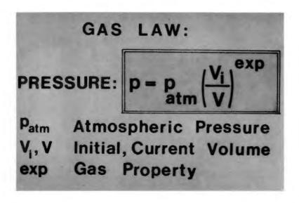
B27. Measurements of combustion chamber pressure have shown that there is normally a delay between ram impact and ignition. This delay time can vary depending on job conditions. It is usually about one or two milliseconds. During this time the impact induced wave is traveling down the pile and the combustion chamber pressure is about constant.
