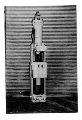
B7. The double acting air/steam hammer has a similar appearance but some important differences in operating characteristics. Of the various types of double acting air/steam hammers, the differential acting type will be described. The main components of this hammer are the same as the single acting machine. The differences are in the configuration of the cylinder. The piston has three surfaces which are subjected to gas pressure, the upper and lower surfaces of the upper
