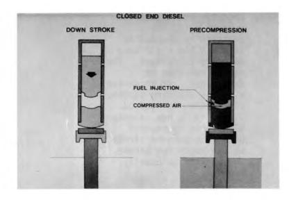
B33. At the bottom of the stroke the ram impacts with the anvil driving is and the pile top down. The bounce chamber ports are cleared and the bounce chamber pressure comes to atmospheric. Ignition occurs at about the same time. The ram then moves upward due to the action of both the pile rebound and the combustion chamber pressure.
