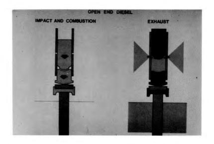
B19. However, the ram has an upward velocity so it continues upward in a free fall condition, in the process drawing in fresh air in a scavenging phase. The maximum height that the ram achieves depends on the pile rebound as well as the combustion effect. In normal operation the stroke can vary over a wide range depending on the pile rebound and stiffness. Strokes ranging between four feet and nine feet are not abnormal for various hammer types.
