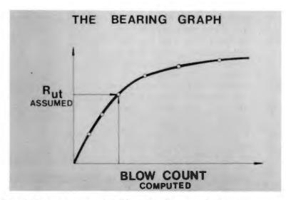
equation analysis is performed and the permanent pile displacement is calculated. The bearing graph is constructed from a set (say 5 or 6) of these points by interpolation.
