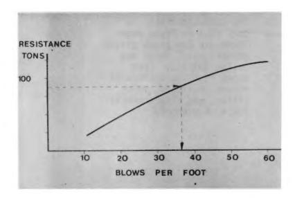
C19. Also plotted in this slide are the stroke results corresponding to the blow counts of the summary. The expected stroke for 90 ton resistance and 36 blows per foot is about 5.8 feet.
