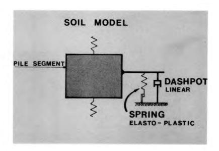
Al7. The spring or static portion of the resistance relates the soil resistance to the pile element displacement. The soil resistance force is assumed to increase linearly with the displacement until a displacement called the quake is reached. With further displacement the force remains constant. Unloading occurs along a line parrallel to the loading line.
