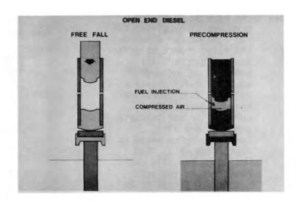
B17. The ram is shaped so that at impact a small combustion chamber remains with a high compression ratio. If the fuel is injected as a liquid it is atomized on impact. Combustion occurs causing a very rapid increase in pressure.
