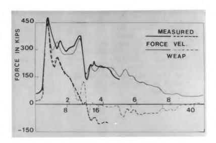
C36. As a third example consider a pile driven by a closed end diesel hammer, the Link-Belt 660. The pile was a 43 foot long pipe of 12-3/4 inch outside diameter. It was driven into very dense silt and sand.
