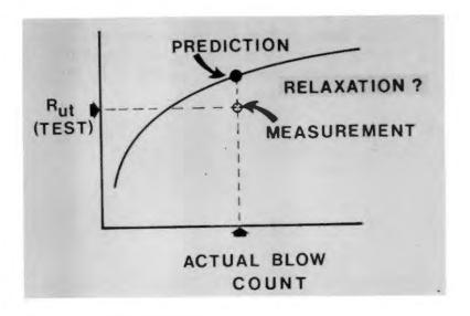
C28. The dynamic soil constants may be incorrectly estimated. The driving system constants may not be correctly known and the hammer performance may not be as expected. Thus, a very large number of constants can be adjusted to achieve a satisfactory correlation with capacity. The value of these constants are certainly not unique.
