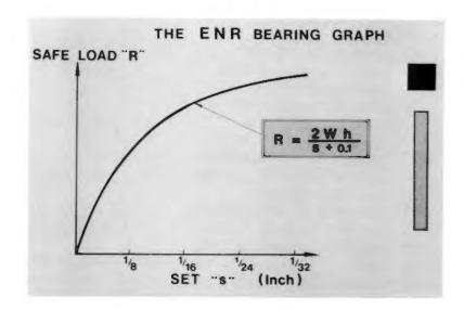
A9. Alternatively, for a specified capacity the required blow count can be determined. Also, an equipment selection can be made. For example, a particular system can only overcome a certain maximum resistance. At the upper range of the curve, a large change in blow count does not indicate a comparable change in capacity.
