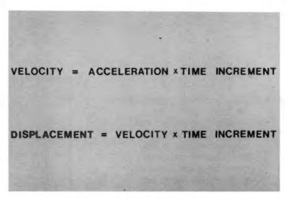
computational effort is increased. The cycle is completed by the determination of the compression in the spring between neighboring elements from the calculated element displacements. The compression then can be converted to forces acting on the elements and the computation repeated for the next time increment.
