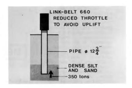
C37. The results are shown here as before. This hammer uses atomized fuel injection, thereby producing an earlier ignition and a smoother transition between precompression and impact on the force record. Again, excellent agreement is achieved.
