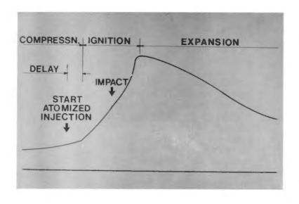
B39. The computer program for the closed end diesel hammer must operate somewhat differently than for open end hammers. If the open throttle stroke is such that lift off is induced then the combustion pressure, associated with a reduced throttle, must be found so that lift off is only incipient. On the other hand, if lift off does not occur then the computation is the same as for open end hammers where the stroke must converge.
