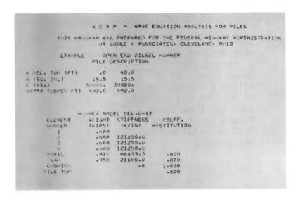
C17. On the last page a summary is printed containing the ultimate resistance, RULT, analyzed, and the corresponding blow count, stroke, minimum and maximum stresses and the speed of the hammer in blows per minute.
