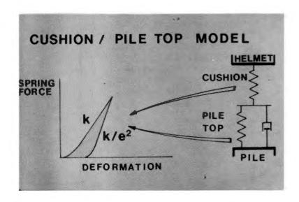
B47. The pile is modeled as a series of masses, springs, and dashpots. The complete model of the pile is shown here. Probably the pile is the simplest element in the total Wave Equation Model. Dashpots have been included to account for some structural damping especially for pile materials like timber.
