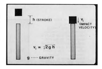
A24. where the stroke is dependent on driving resistance and is not known in advance. Difficulties have been encountered, particularly with the stress predictions obtained from these programs.
