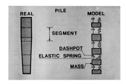
B48. The soil model was already introduced in the first section of this presentation. It consists of an elasto plastic spring which reaches an ultimate resistance force at a compression value called the quake.
