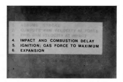
B28. When ignition occurs the pressure increases very rapidly to some maximum value. This pressure can be calculated from combustion laws. However, due to the imperfect nature of diesel hammer combustion the computed pressure is not reliable. Therefore, measured maximum pressures are used in the WEAP program. From this time on the combustion chamber pressure used in WEAP is determined by the volume of the chamber using the gas law.
