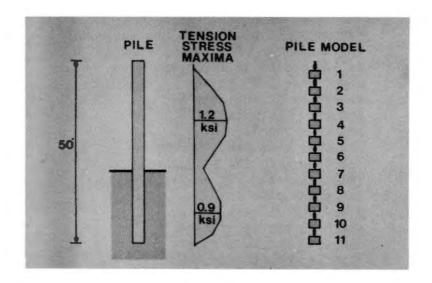
C24. Thus the tension stresses are too high. A rerun of this problem with 6 cushion sheets and, therefore, a cushion stiffness which is only 1680 kips/inch, produces a tension stress of 0.6 ksi.
