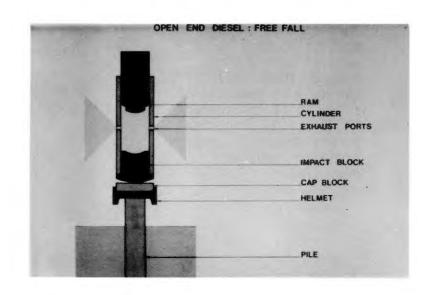
B16. When the ram falls past the exhaust ports they are blocked and the precompression phase begins. The falling ram activates a cam to inject fuel into the cylinder. This may be in liquid form falling onto the impact block or it may be atomized. In the latter case it is injected only shortly before impact.
