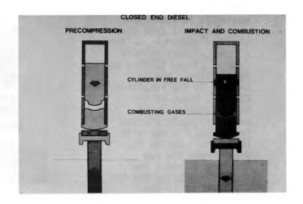
B34. When the exhaust ports are cleared the combustion chamber goes down to the ambient atmospheric pressure. Also, a pressure is built up in the bounce chamber slowing the ram down more quickly than would gravity alone.
