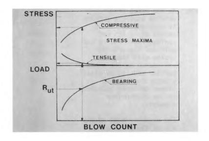
A21. It should be noted that a bearing graph is associated with a particular pile penetation. While it is similar in appearance to the graph generated by a dynamic formula, it represents something quite different. The dynamic formula has as its only variable, hammer energy with, perhaps, an estimate of losses. The wave equation includes pile flexibility, an estimate of soil perfor-
