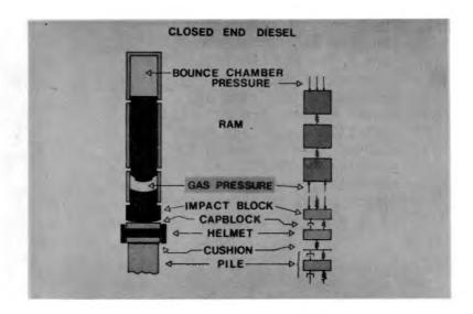
B25. The program begins with either an assumed or a user specified ram stroke. With a knowledge of the stroke the velocity of the ram as it falls past the exhaust ports can be calculated from elementary kinematics. When the exhaust ports are closed the combustion chamber pressure and ram velocity are determined using a rigid body assumption and step-wise calculating ram velocity resulting from the action of gravitational and combustion forces.
