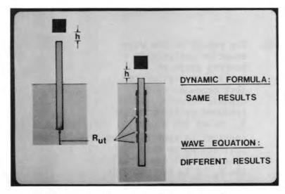
mance, and driving system characteristics. In the case shown here the dynamic formula would give the same bearing graph in both cases while the wave equation bearing graph would be different.
