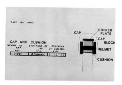
C12. Coefficients of restitution are left blank on card no. 4 except for the capblock where a 0.8 is inserted as appropriate for conbest. The computer will make a reasonable choice for all quantities that are left blank on this card.
