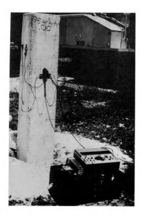
C30. This huge volume of data (several thousand hammer blows) was available to test the program. The available measurements consist of force and acceleration records at the pile top. These measurements were compared with the values obtained by WEAP. One of the major activities of the project was to provide recommendations on the values to be used for the hammer dynamic constants. Sixteen different jobs were so tested and the results are presented in the final
