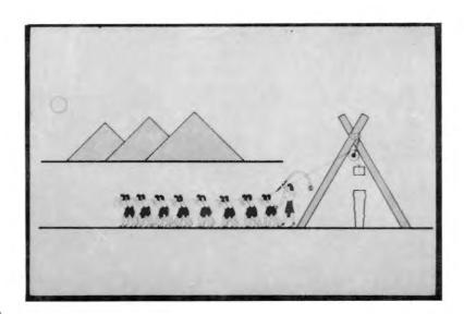
A3. Probably, failure of the pile or the driving operation was a common occurrence. During the last century pile usage increased with the development of the single acting steam hammer.
