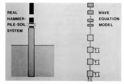
system including the soil. Computer programs have been prepared to perform the analysis and these programs have come to be known as Wave Equation programs. In this presentation the name wave equation will refer to computer programs of this general type.
