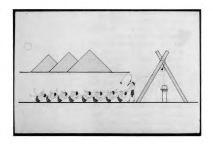
A4. Methods for predicting pile strength were proposed using dynamic data obtained during driving. Since the only realistic measurements at that time were ram stroke and pile set (or blow count)
