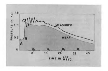
attempt is made to represent it. It can be seen that the pressure calculated by WEAP is similar but somewhat smaller than the measured value.
