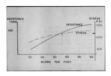
C21. A second type of wave equation application is for the control of tension stresses in concrete piles. As an example consider a Vulcan 80C differential acting air/ steam hammer driving a 50 foot long, 14 x 14 inch square, prestressed concrete pile. The soil overlaying the bearing strata is very soft and a situation is to be analyzed with only 10 tons skin resistance and a Smith skin damping value of 0.2 at a penetration of 20 feet. The cushion thickness is to be
