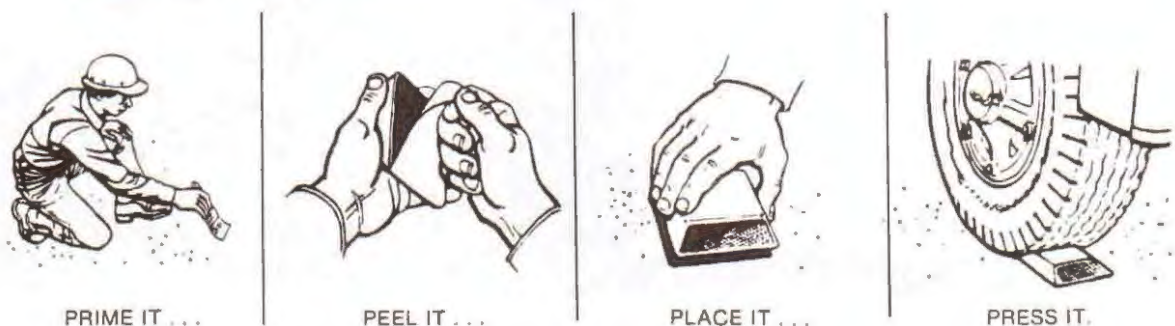
Figure 38. Application of Pressure Sensitive Reflective Raised Marker
