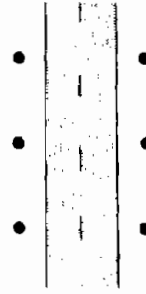
Utility pole placement on both sides.
