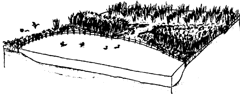
A site may be protected against waterfowl depredation by installing an inexpensive nylon line fence. More substantial fences may have to be used to exclude larger animals.
