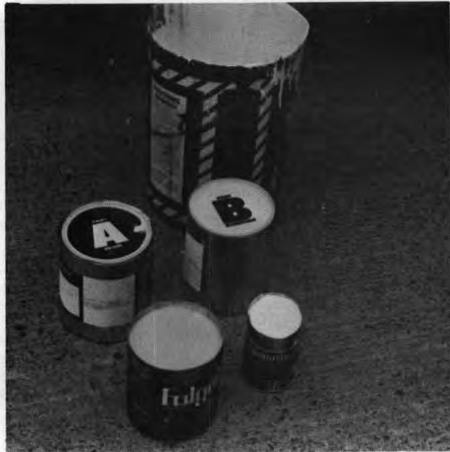
Figure 11. Two-part Concrecive 1064 components, glass beads, and 5-gallon mixing bucket.
