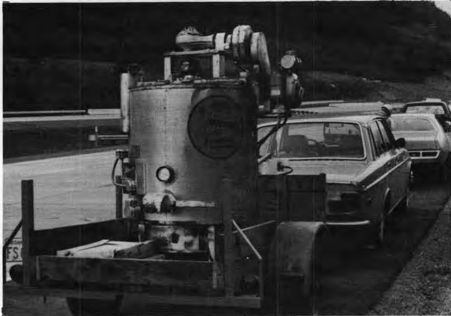
Figure 9. Trailer-mounted heating vat for liquifying Cleanosol. Solid ingots of Cleanosol are visible in the cardboard boxes behind the heater. The applicator machine is filled from the dispenser on the rear of the vat.
