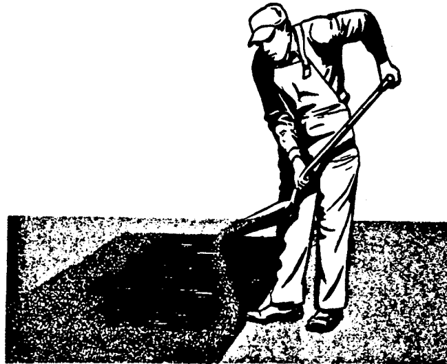
FIGURE 3.29 STEP 4. SPREAD AGGREGATE
