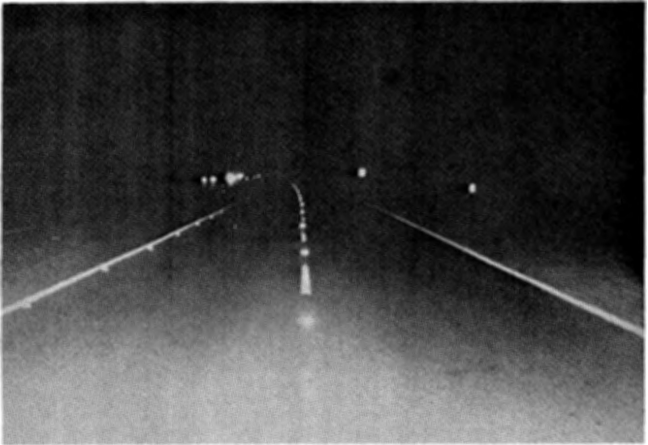
Figure 7. Photograph Taken in December 1980 at the Jessamine County Southbound Installation (Pattern of Markers is Recessed, Dura-Brite, Stimsonite 96, and Kingray).
