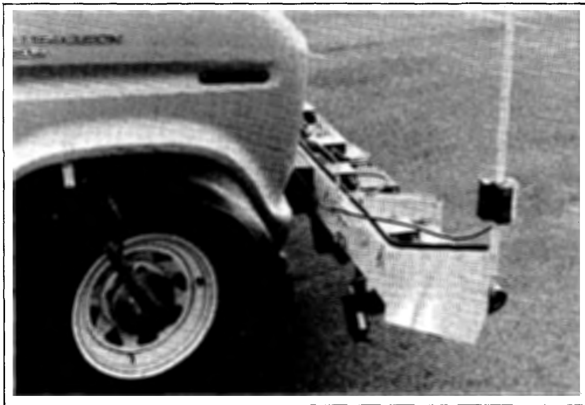
Figure 23. Side view of IMS Laser RST (top) and laser support beam and distance recorder (bottom).
