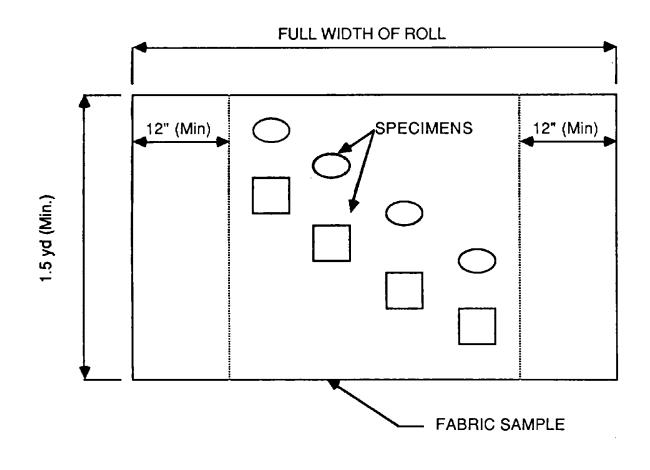
Figure 1 - Test Specimen Selection
