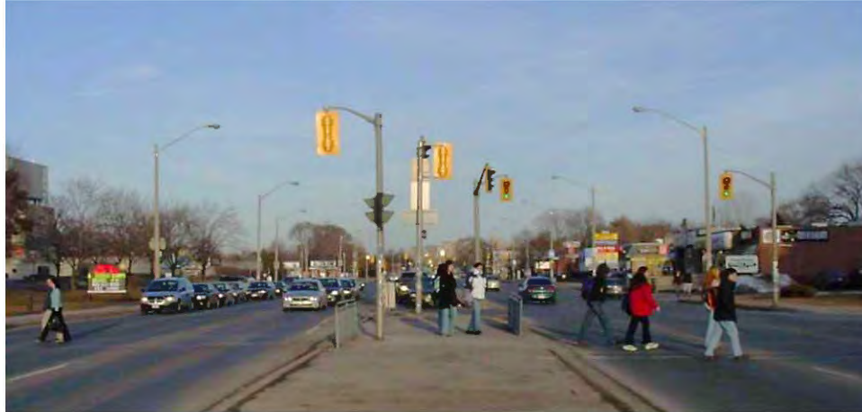
Figure 61. This refuge island enables two-stage pedestrian crossings.
