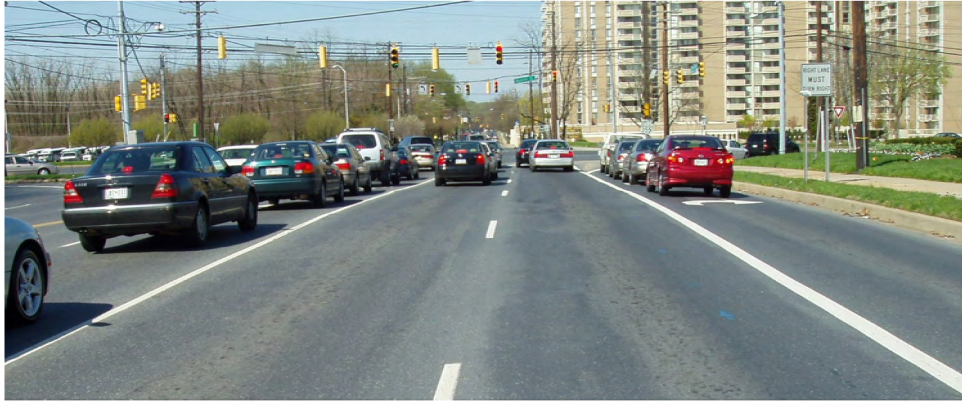
Figure 123. Narrow (2.4-m (8-ft)) right-turn lanes may be used effectively in retrofit situations.
