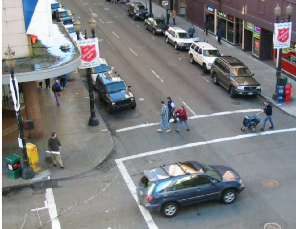
Figure 8. Crosswalks are used by a variety of users with different speed characteristics. Pedestrian walking speeds generally range between 0.8 to 1.8 m/s (2.5 to 6.0 ft/s).
