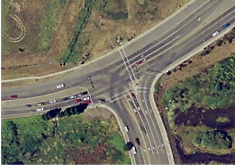
Figure 14. The photo shows how double left-turn and double right-turn lanes can be used to accommodate high-priority movements.
