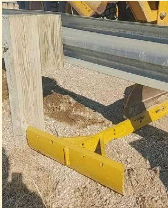
The Guardrail Maintainer, an innovation by North Dakota’s Walsh County Highway Department, was one of four winners of the 2022 Build a Better Mousetrap competition.
