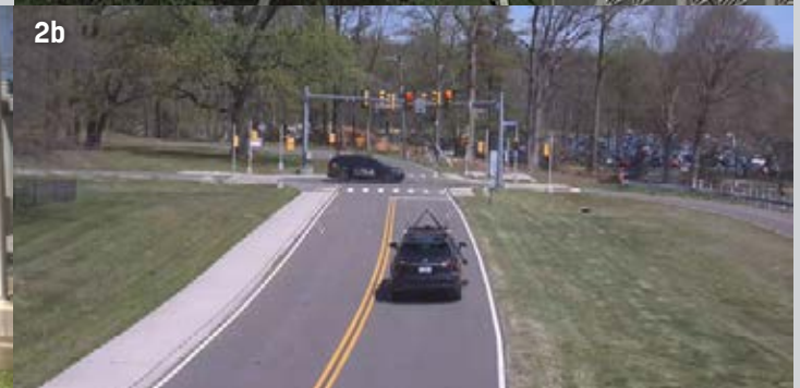
2b. Use case 2: A vehicle adjusts its approach to entering an intersection where it receives a red (stop) signal indication as a second vehicle receives a green (go) signal indication. The first vehicle will come to a stop if the red signal indication continues.
