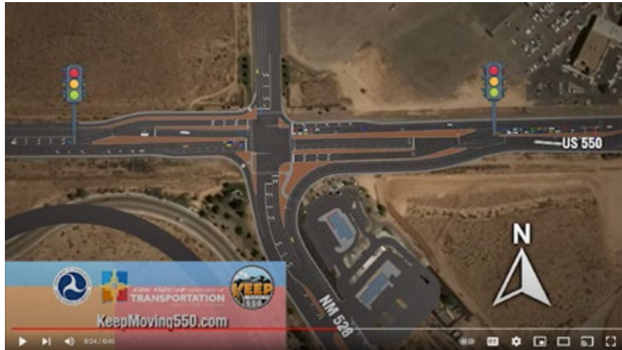
Screenshot from an educational video NMDOT published to help drivers understand how the State's first continuous flow intersection works.
