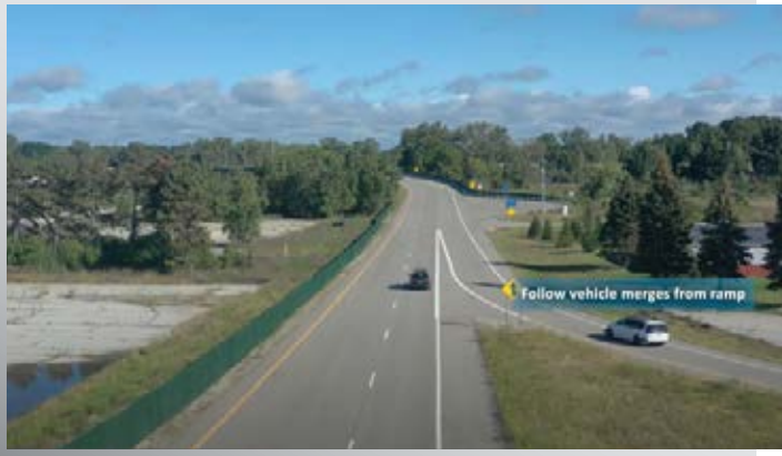
CARMA Platform-equipped vehicle merges onto a freeway during validation testing. Source: FHWA.
