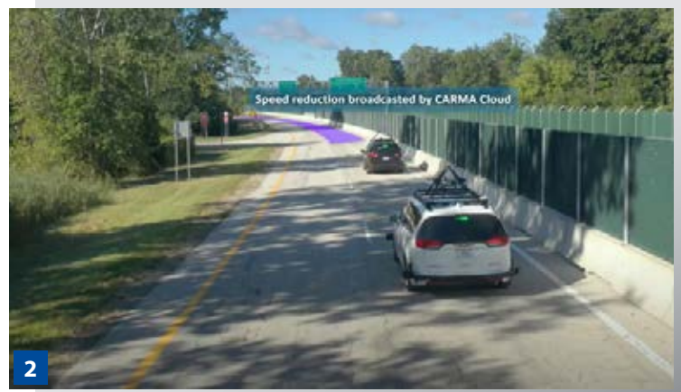
1. Vehicles form a platoon after the merge. 2. Lead vehicle receives speed advisory broadcasted by CARMA Cloud.
