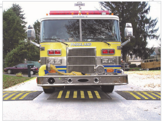
Speed management countermeasures for residential streets may include speed cushions like these, which calm vehicle traffic but include wheel cutouts that allow fire apparatuses to bypass in case of emergency response.
