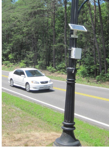
Figure 3. Sensor mounted to county-owned infrastructure
