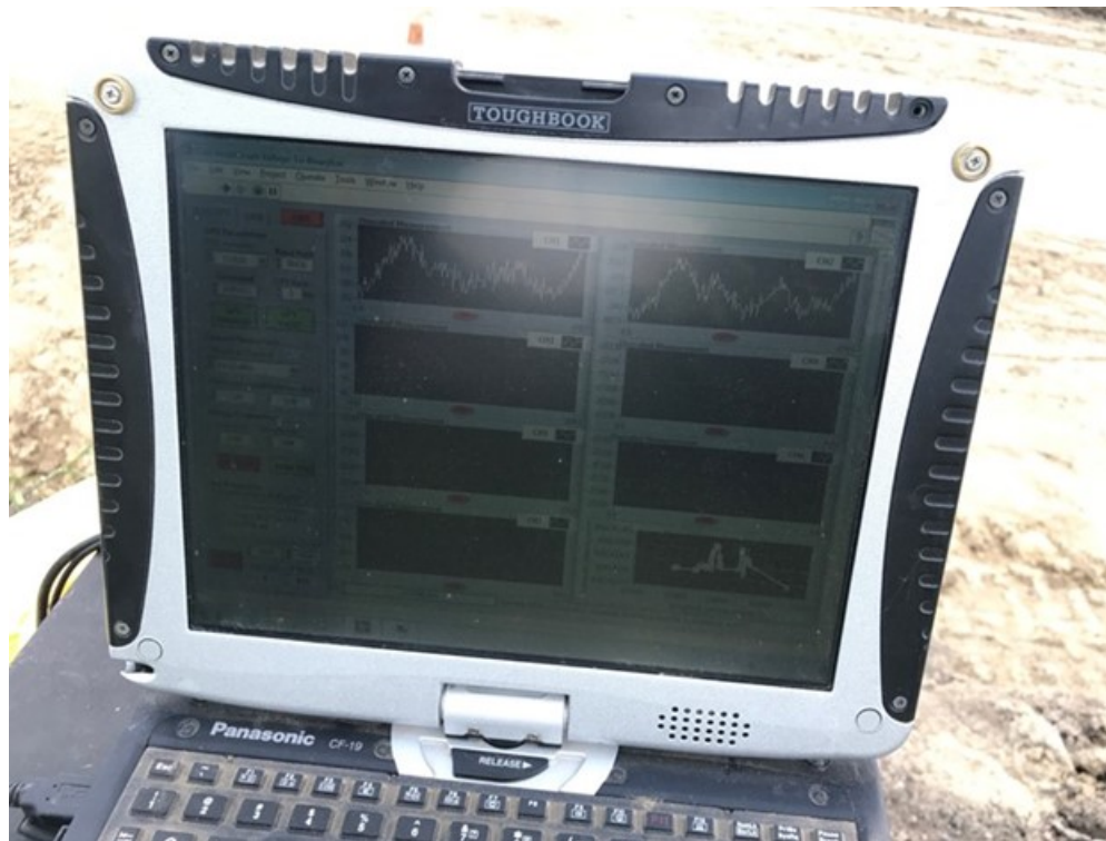
Figure 17. Monitoring of the geophone signals for IC data calibration.
