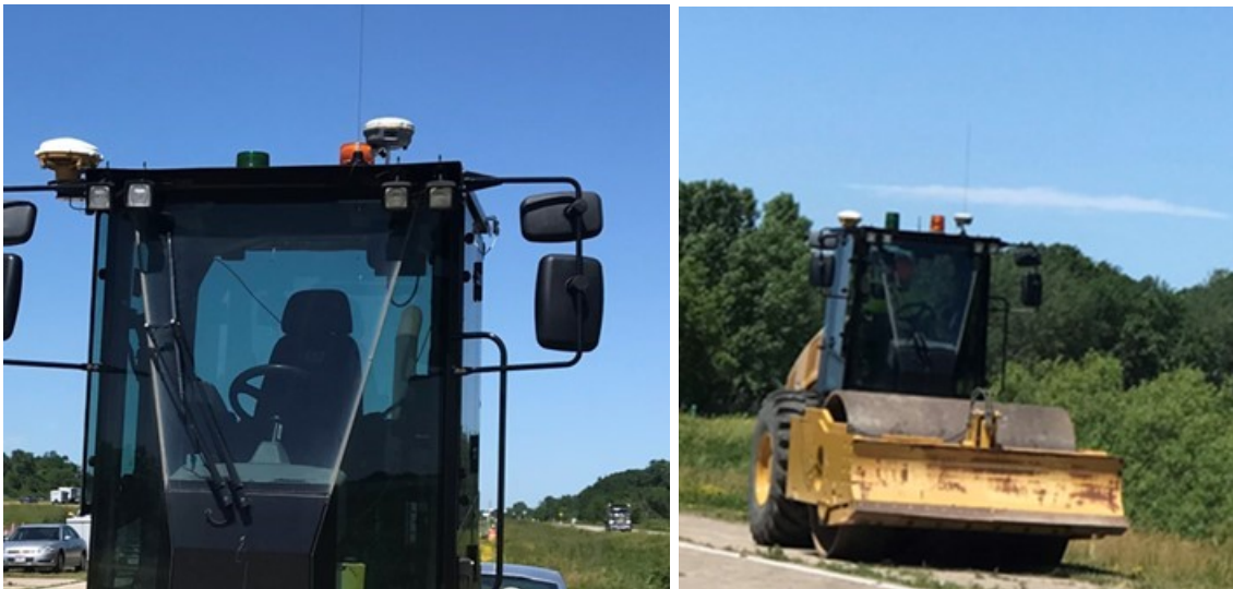
Figure 9. UTEP Moduli ICMV GPS (left) and fully-instrumented roller (right).
