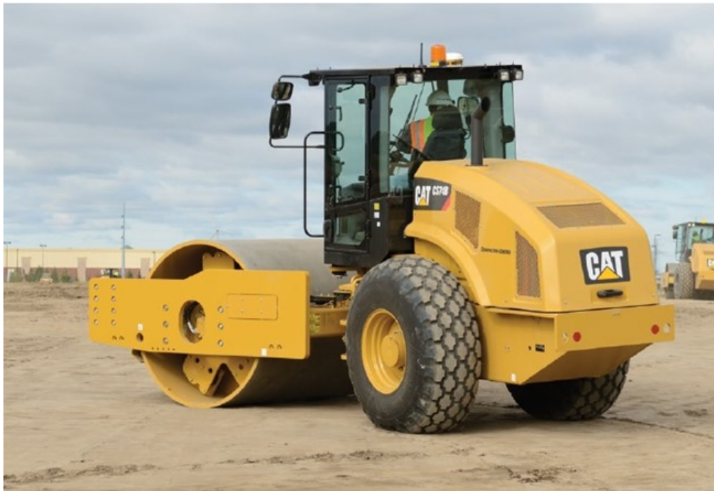
Figure 4. A single smooth drum IC roller (Caterpillar Model CS74B).
