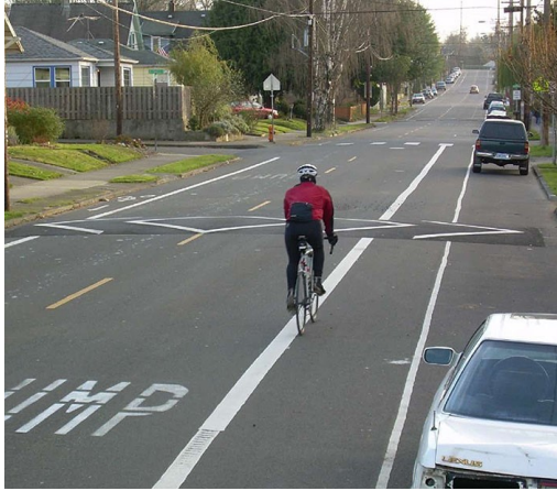
Figure 2.13 Speed hump. (Source: FHWA)
