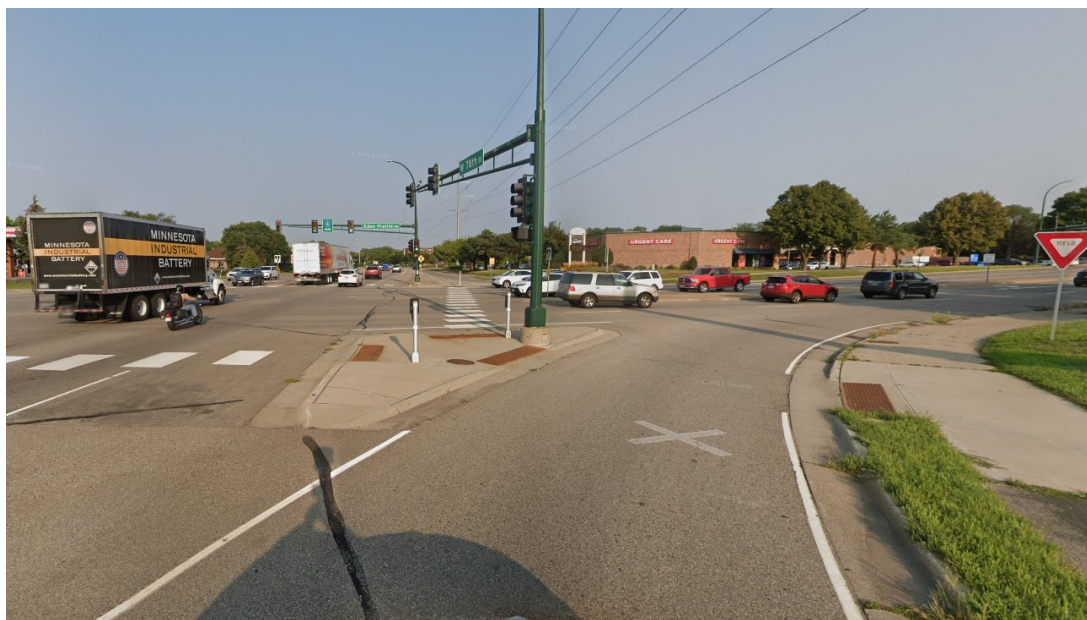
Figure 2.10 Typical slip lane and porkchop island, Arboretum Blvd/78th Street (MN 5) at Eden Prairie Road, Eden Prairie, MN. (Source: Google StreetView)
