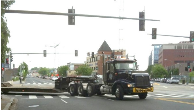
Figure 2.6 Right-turning truck encroaching adjacent lanes. (Source: National Association of City Transportation Officials)
