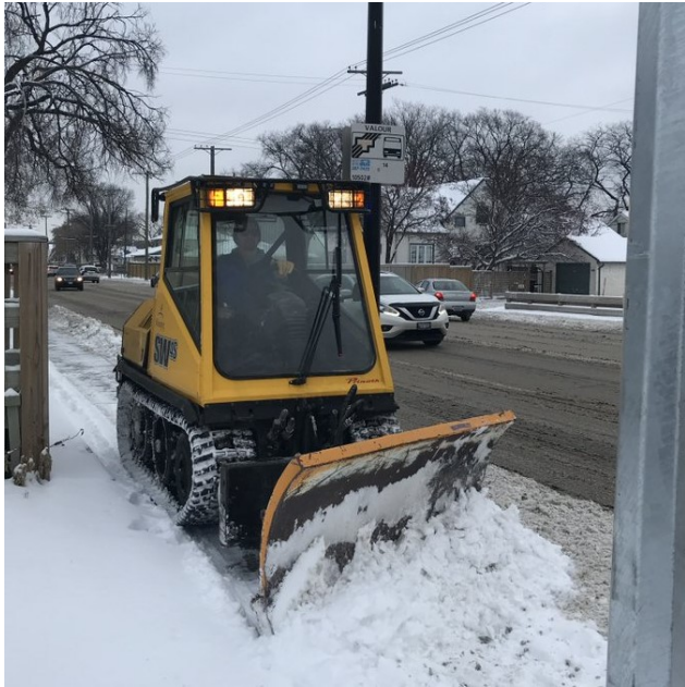
Figure 4.4 Sidewalk snow removal in Winnipeg (Source: City of Winnipeg/Twitter)
