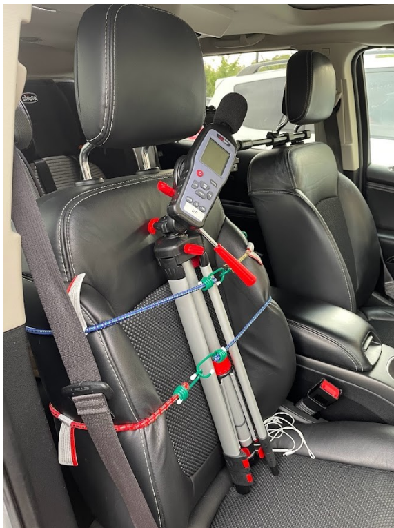
Figure 4-6. Interior noise test setup
