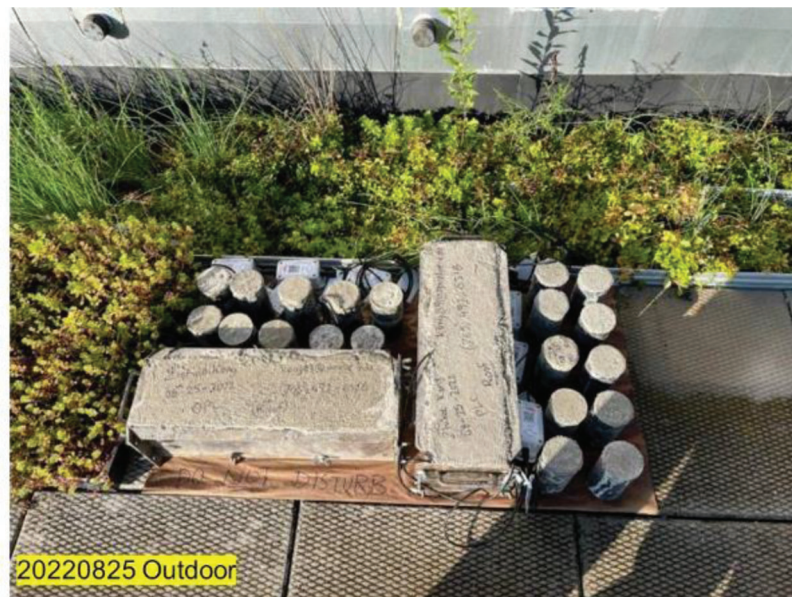
Figure 4.10 Concrete samples cured outdoors.
