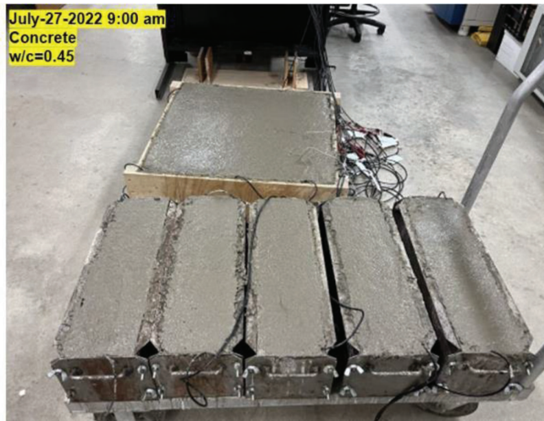
Figure 4.8 Concrete beams and slab casted in the lab.
