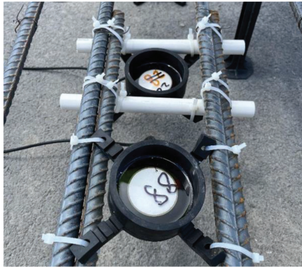
Figure 5.12 Sensor placement of I-35E field testing.
