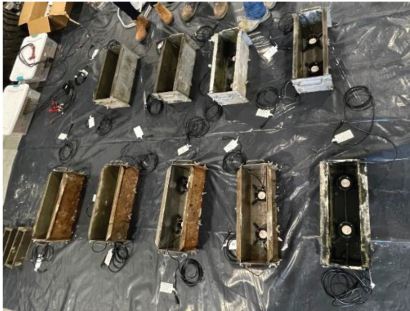
Figure 5.8 Sensor placement in beams of Shelby field testing.
