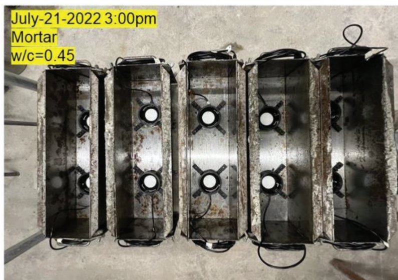
Figure 4.1 Sensor placement in beam molds.
