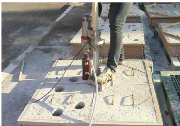
Figure 2.2 A typical core drilling setup (Ju et al., 2017).
