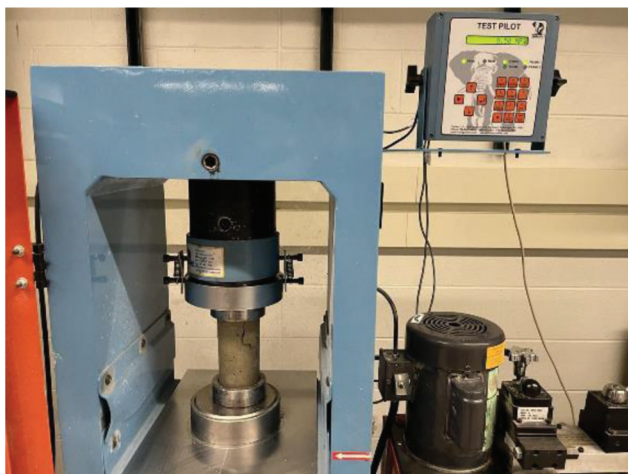
Figure 2.1 A typical compression testing setup.
