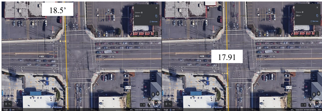
Average Setback Distance Measurement at Lancaster Dr. NE and Market St. NE
