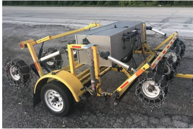
Figure 3.4 Automated sounding system from Consultant A (used with permission from consultant).
