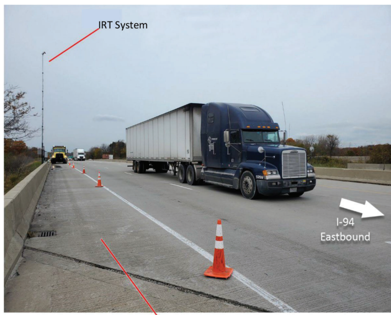
Figure 3.24 Typical top deck equipment setup on the barrier rail (used with permission from consultant).
