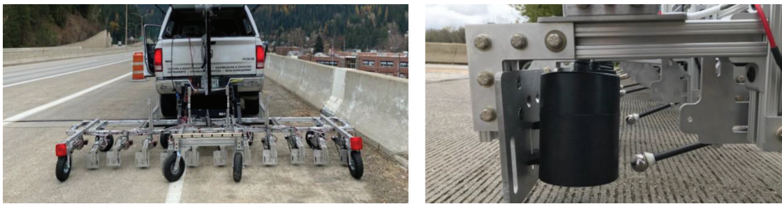
Figure 3.5 Automated sounding system (left); individual impactor and microphone (right) (used with permission from consultant).
