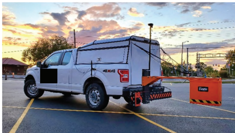
Figure 3.22 GSSI RoadScan 30 system (used with permission from consultant).
