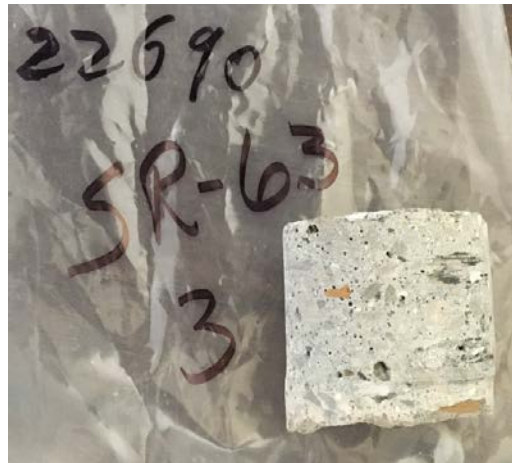
Figure B.3 Photos of the concrete cores for Bridges 22690 (First Round).
