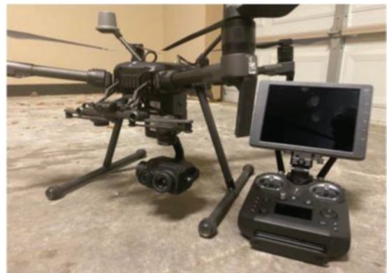
Figure 2.7 Example of drone-mounted IRT equipment (used with permission from consultant).
