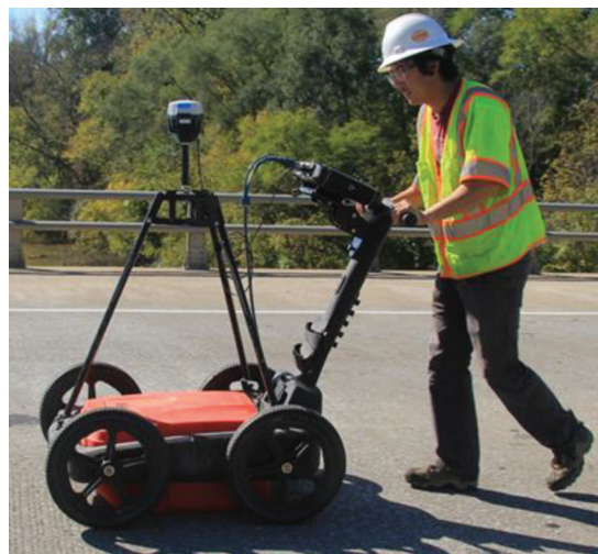
Figure 3.21 Ground-coupled GPR equipment from Consultant F.
