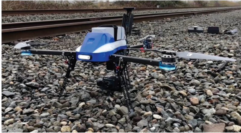
Figure 3.7 Photo of a FLIR Duo Pro R 640 Thermal Camera/13 mm/30 HZ mounted on a Switchblade-Elite drone (used with permission from consultant).
