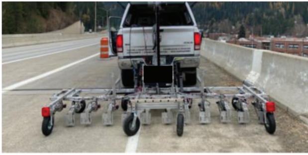
Figure 2.3 Example of equipment for automated sounding inspection (used with permission from consultant).
