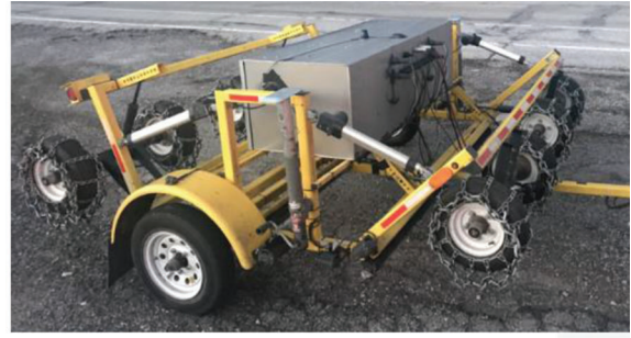
Figure 2.3 Example of equipment for automated sounding inspection (used with permission from consultant).
