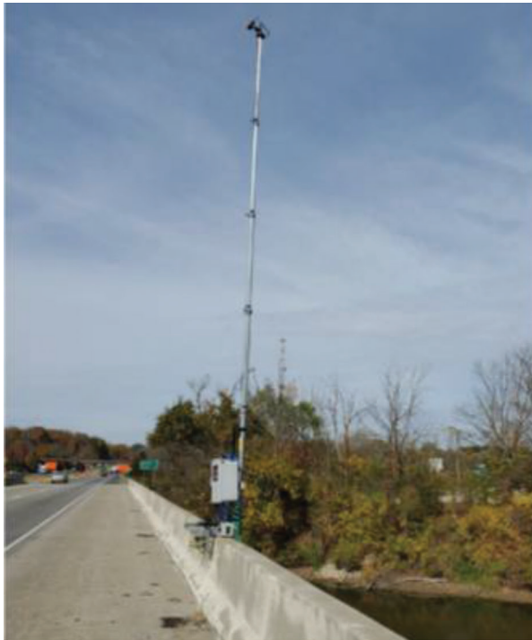
Figure 2.8 Example of pole-mounted IRT equipment (used with permission from consultant).
