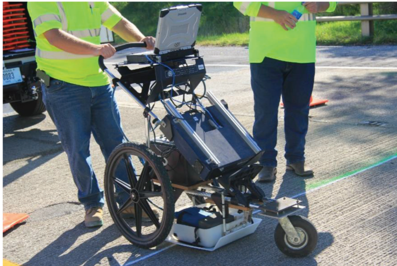
Figure 3.10 Ground-coupled GPR equipment used by INDOT.
