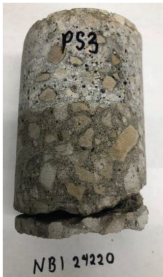
Figure 2.9 Example of a concrete core.
