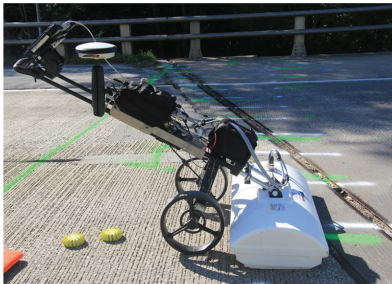
Figure 3.23 Ground-coupled MCGPR equipment (IDS GeoRadar RIS Hi-BrigHT).
