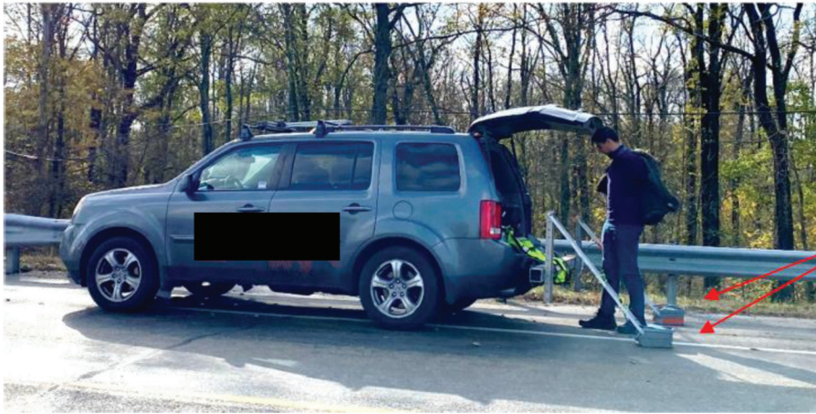
Figure 3.13 Ground-coupled PL GPR survey—antenna mounting to vehicle (used with permission from consultant).
