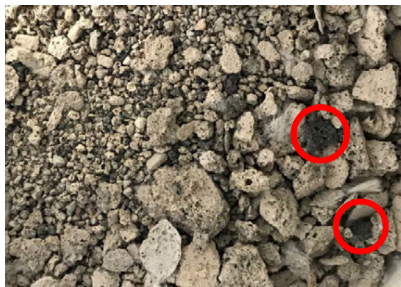
Unburned asphalt remains after an ignition test performed at 800°F for RAS material.
