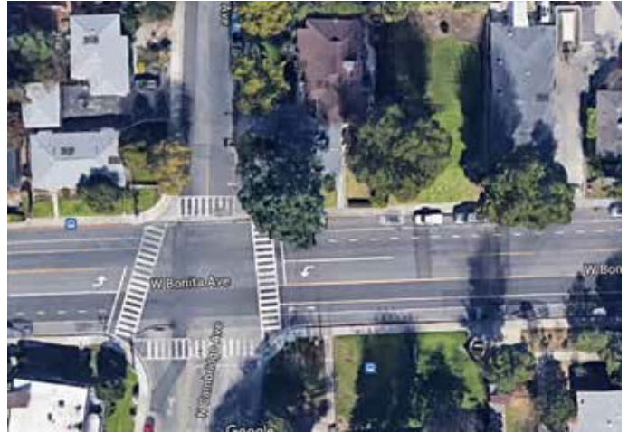
Well-marked pedestrian crossings with signal at intersections on Bonita Ave leading to transit stop. Bonita also includes a bike lane.
