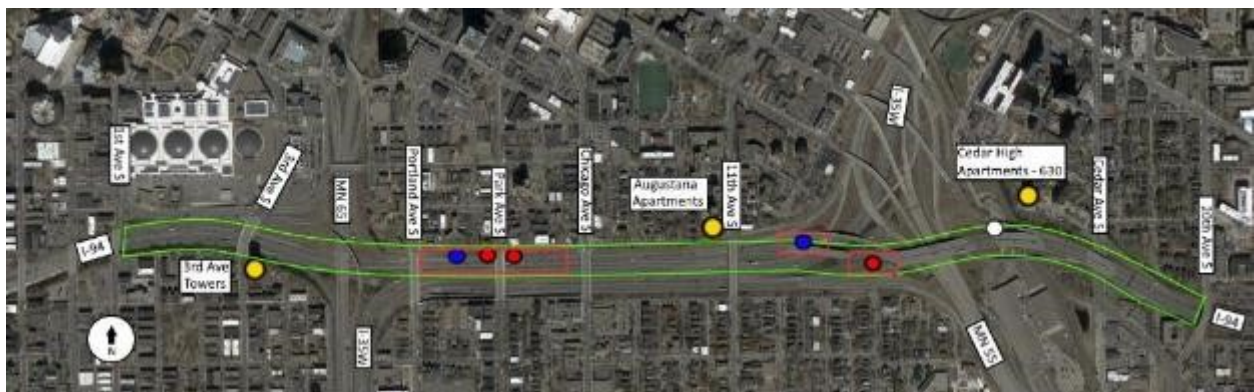
Figure 3-2 New Field Lab site showing radar sites (red dots), Wavetronix sites (blue dots), radar coverage (red outlines), rooftop stations (yellow dots), and a future MnDOT station (white dot).
