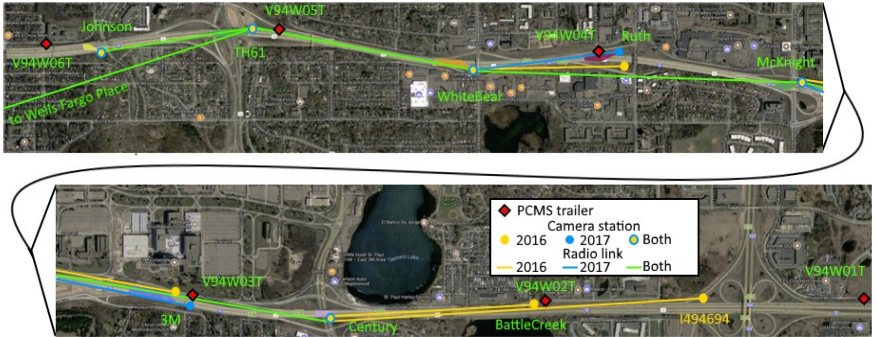
Figure 1-8 SWZSN Work zone with PCMS trailers, camera stations, and radio links
