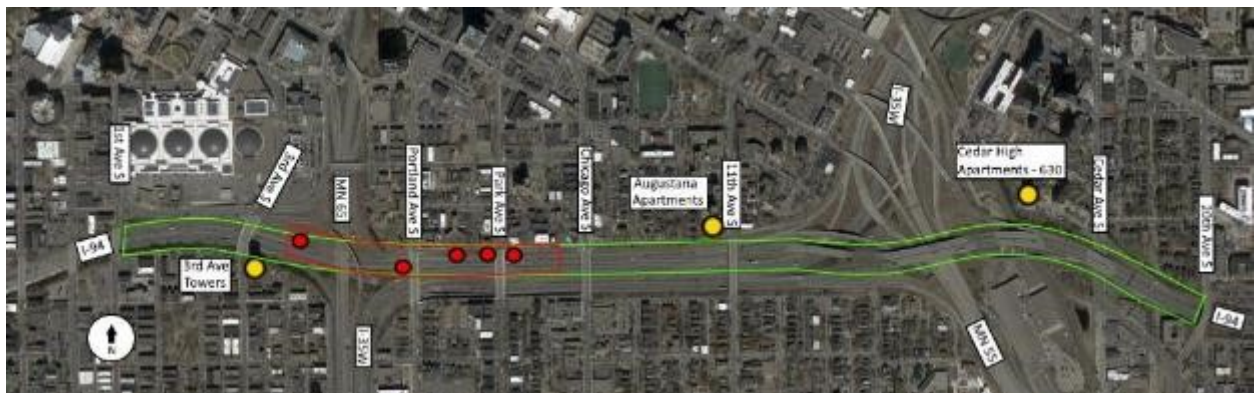
Figure 3-1 Original Field Lab site showing radar sites (red dots), radar coverage (outlined in red), rooftop stations (yellow dots) and camera coverage (outlined in green).
