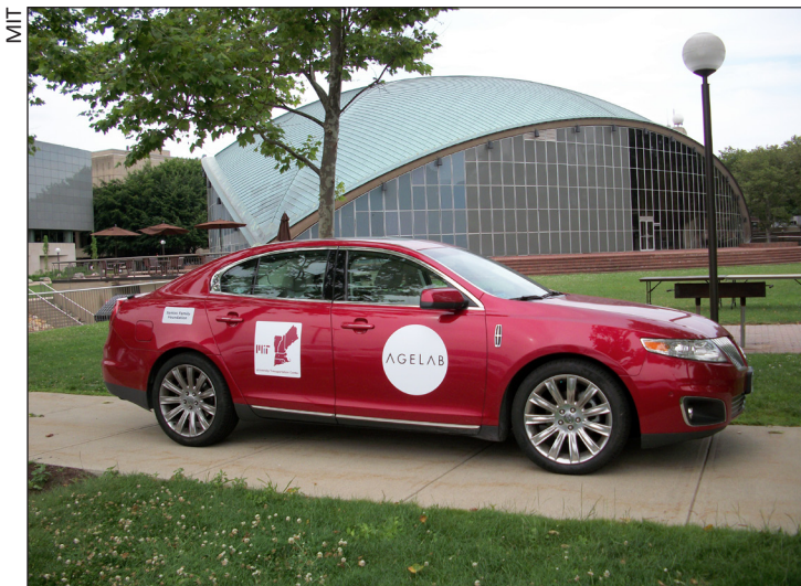
The MIT AwareCar, a specially instrumented vehicle designed to measure a driver's behavior in real-time on the roadway.
