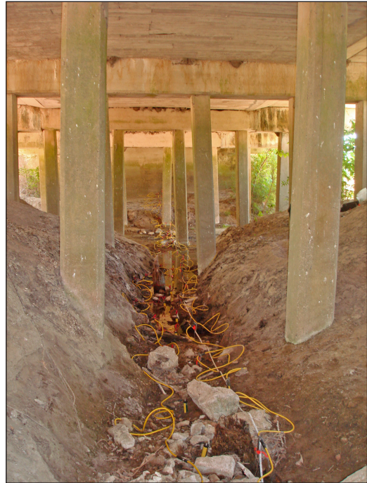
Electrode line array under Gum Creek Bridge in Grimes County, Texas.
