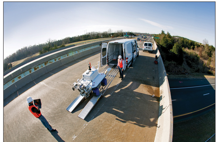
The team deploys the RABIT™ bridge deck assessment tool.
