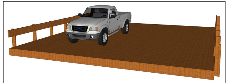
Figure 2. Glulam slab timber bridge. (by: Zach Carnahan)
