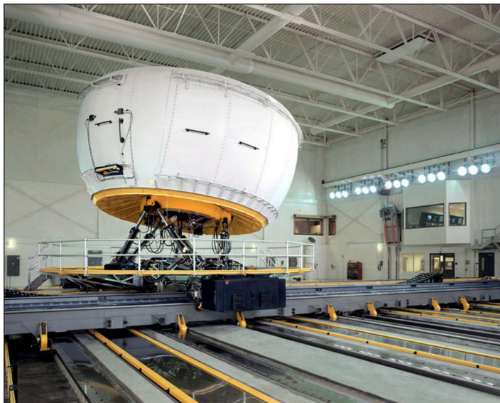
The NADS high fidelity driving simulator is owned by USDOT NHTSA and operated by the University of Iowa.
