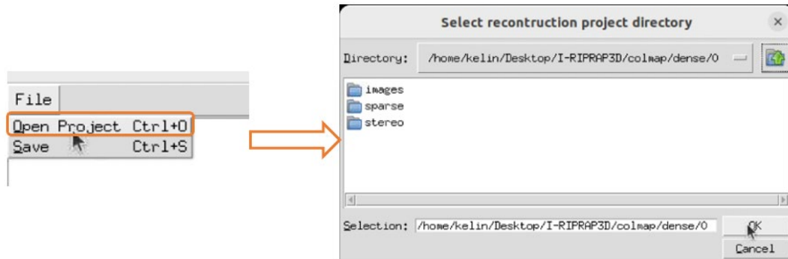
Figure 14. Importing reconstructed project for scale calibration.
