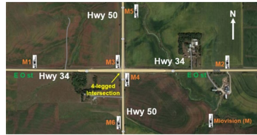
Site 4: Miovision installed in 4-legged non-FRT intersection
