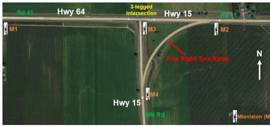
Site 1: Miovision installed in 3-legged FRT intersection
