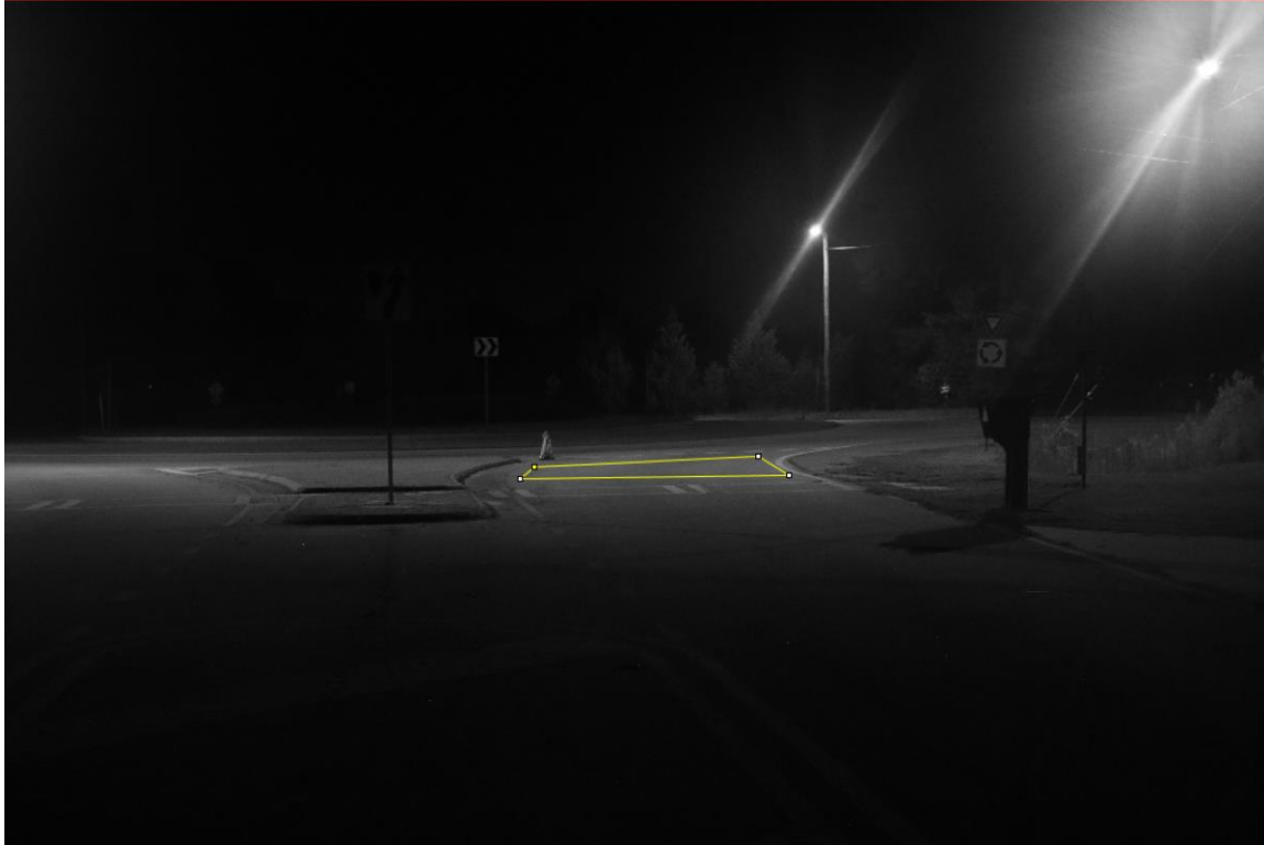
Figure 11. Image. Roundabout Approach with the Luminance Measurement Area Highlighted in Yellow (Tripod-mounted camera image)
