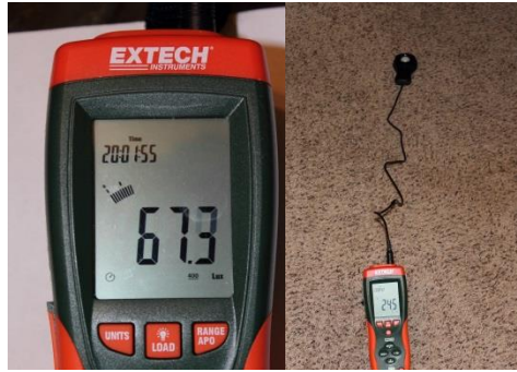
Figure. Picture of the illuminance meter. Left picture shows the screen with the correct illuminance range. Right picture shows the meter with the sensor cable stretched out.
