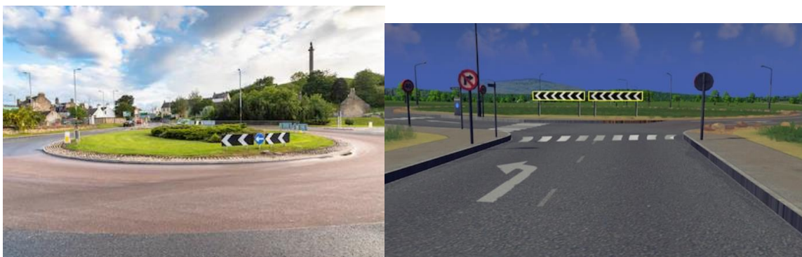
Figure 6. Image. Chevron signs at roundabouts
