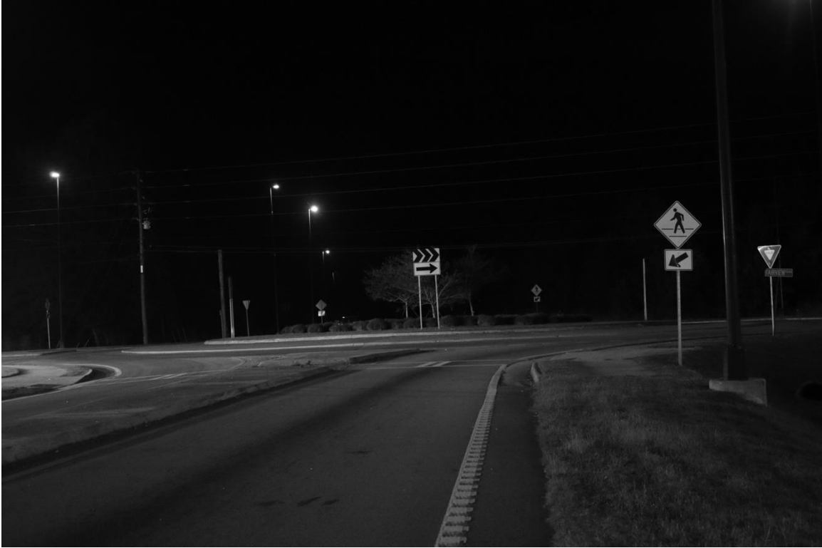
Figure 13. Image. A typical nighttime image of a roundabout taken for luminance analysis with the tripod mounted DSLR camera
