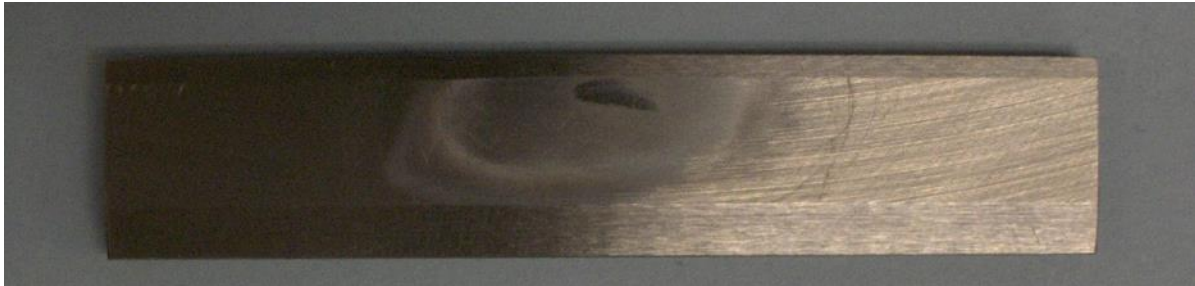
Figure E- 2. Anomaly specimen prior to peening demonstrating unequal width chamfers
