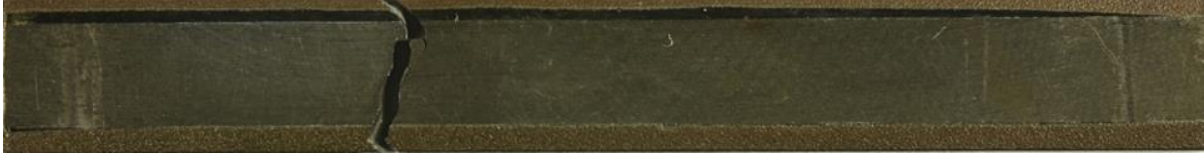
Figure E- 9. MTU IN-718 baseline #2 specimen
