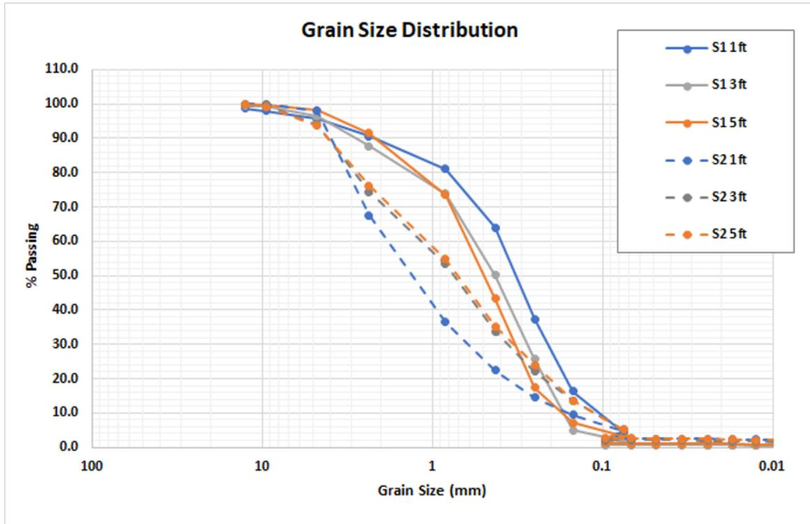
Figure 4. Graph. Grain-size distribution result.
