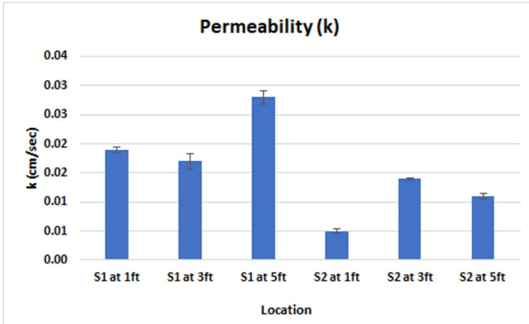
Figure 6. Graph. Permeability of dredged material.
