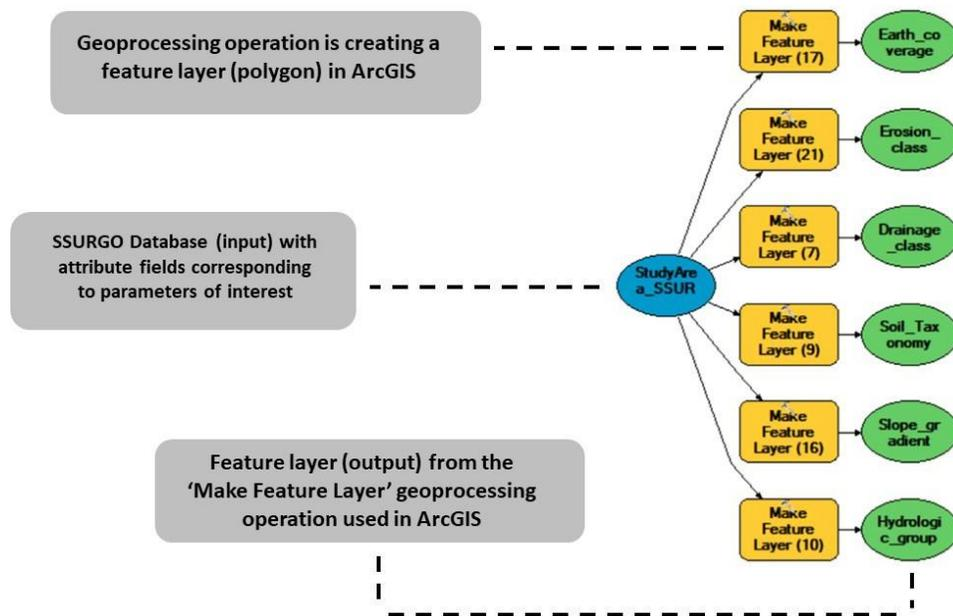
**Figure 10. Diagram. Geoprocessing site model performing spatial queries on selected SSURGO attributes (i.e., site variables) within the Modelbuilder application in ArcGIS 10.4.**
