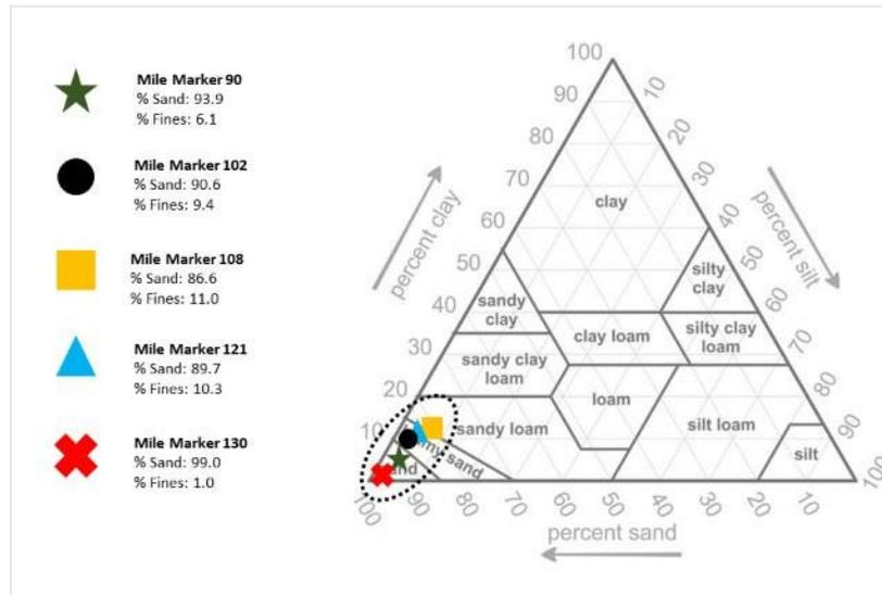
**Figure 12. Diagram. Soil texture classifications for right-of-way sites.**
