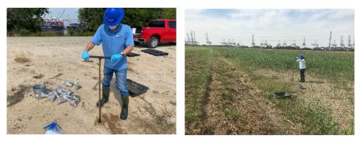
(a) S1 Location(b) S2 LocationFigure 2. Photos. Sampling using a hand auger.
