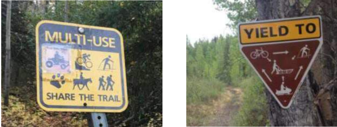
Figure 2.2. Example of signs indicating (a) the nature of and appropriate modes on a multi-use trail and (b) modal-based right-of-ways
