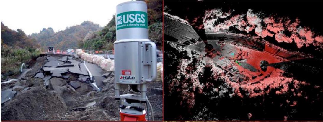
Figure 51. Photo. Terrestrial LiDAR system, including the merge of scans from different positions to accomplish a thorough survey of the failure zone ( Rathje et al., 2016 ).
