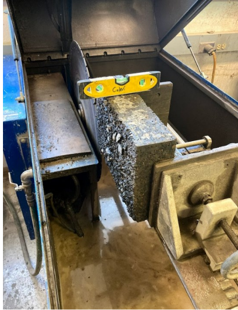
Figure 4.8: Cutting samples using water-cooled diamond blade
