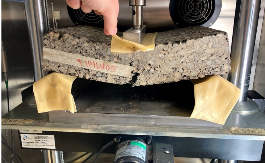
Figure 4.10: Tested three-point flexural fatigue sample
