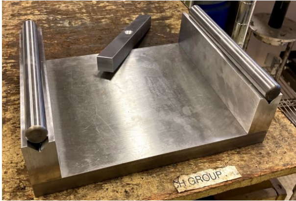
(a) Three-point bending frame developed at OSU
