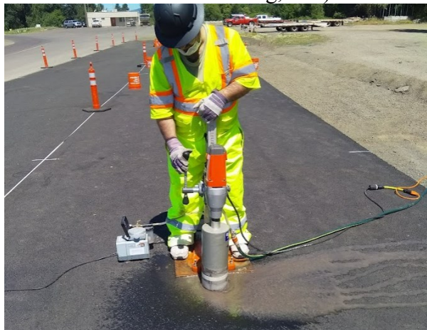
(f) Coring for laboratory density measurement and testing
