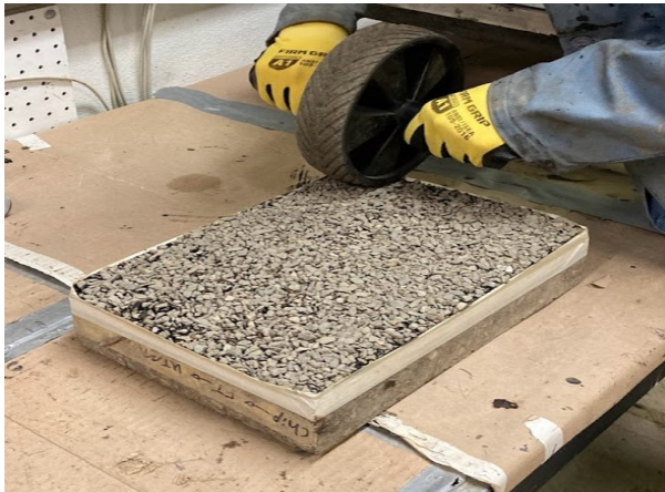
(e) Compacting aggregates
