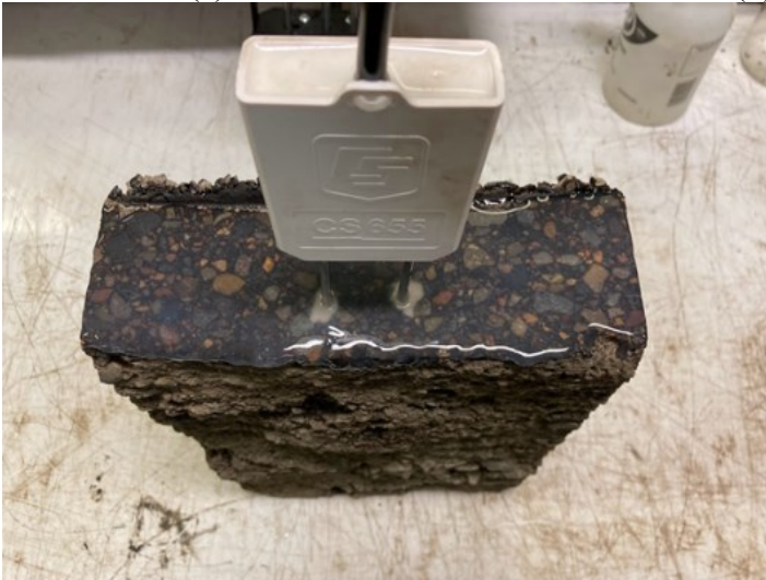
(c) Moisture sensor sealed with silicone gel
