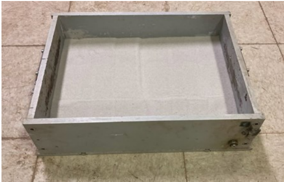
(a) HWTT mold with sand base layer
