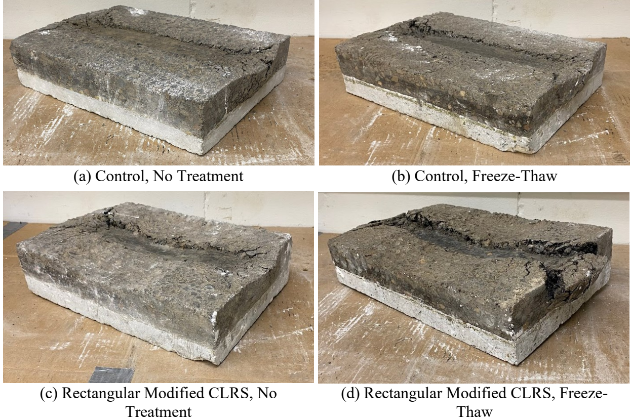
Figure 4.45: HWTT - Cracking patterns after freeze-thaw conditioning
