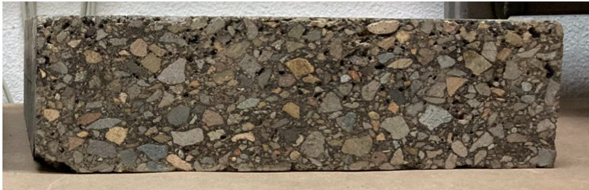
(b) Air voids – Unconstrained edge of the travel lane
