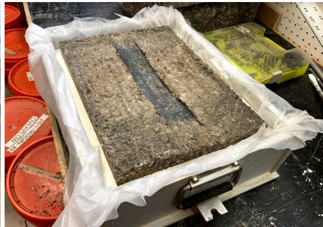
(b) Tested CLRS block sample with cracking
