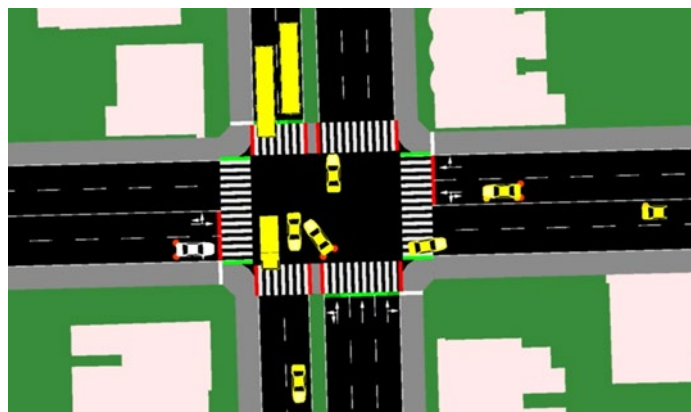
Figure 1. Screenshot from the SUMO traffic simulation software that shows road user intersection behavior.
