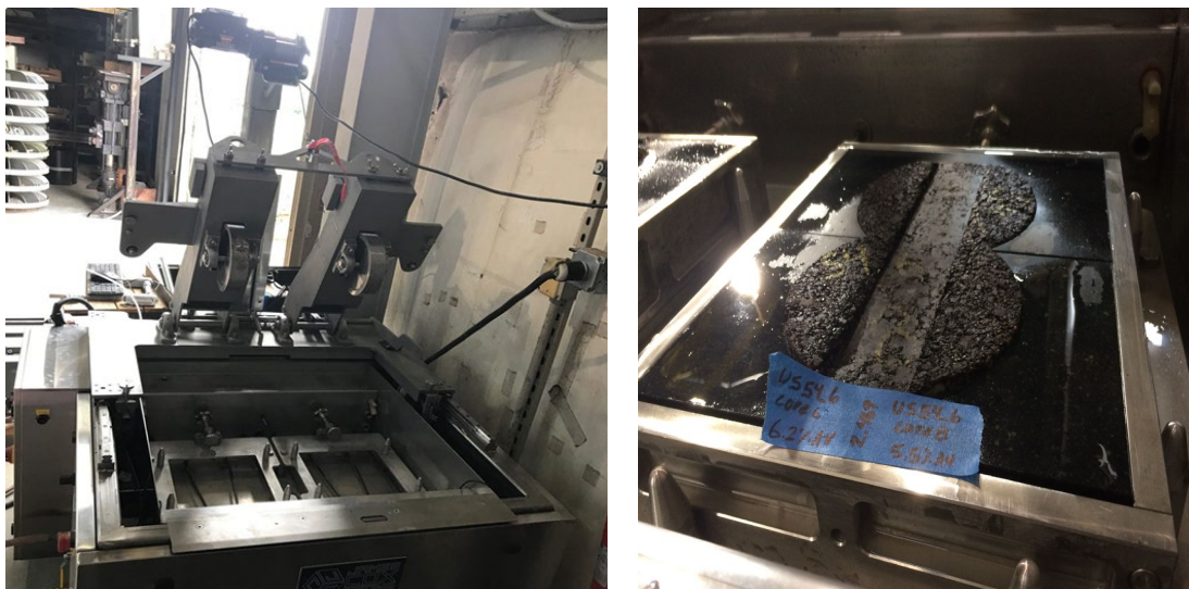
Figure 4-2. Hamburg Wheel Tracking Device: a) Test Device b) Mixtures after test
