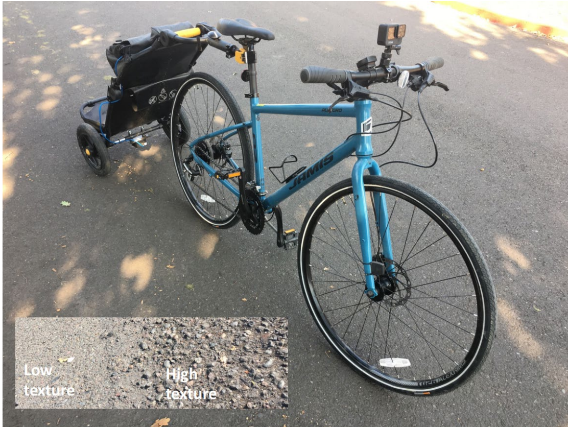
Figure 2-2. Developed bike system with all components with a high and low texture comparison.
