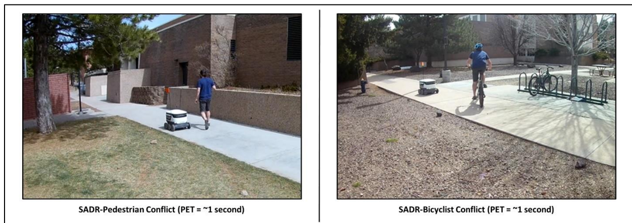
Figure 6. Video screen shot of SADR conflicts in stated choice experiment with pedestrian (left) and bicyclist (right)
