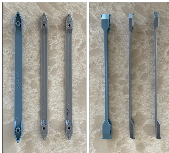
Figure 6. Bridge Members: Original, Moderate Damage and Severe Damage Member (from left to right)
