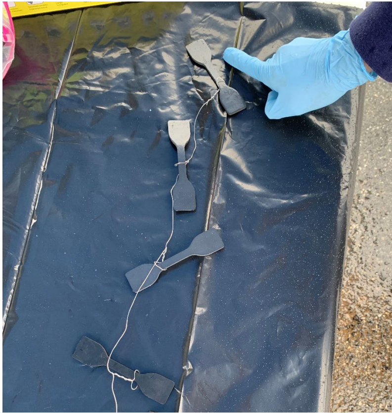
Figure C6. Gasket samples for measuring tensile strength degradation tied together before deployment in the monitoring well.
