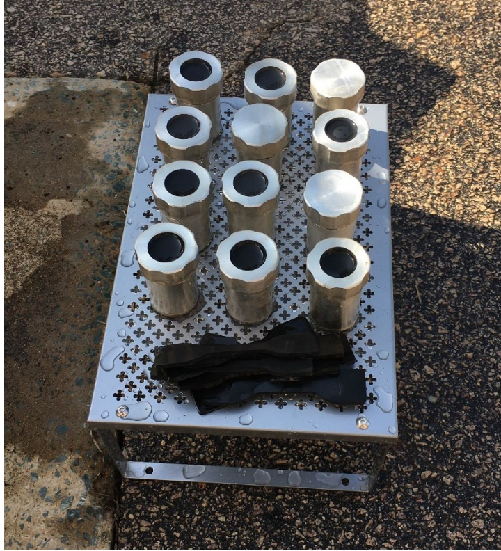
Figure C8. After retrieval from the monitoring wells, capsules and gasket samples were washed on site before transportation to the lab.
