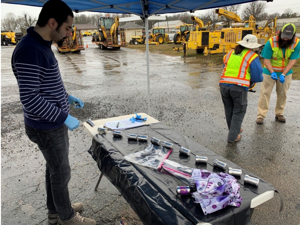
Figure C4. Capsules tied up with stainless steel wire for deployment in the monitoring well.
