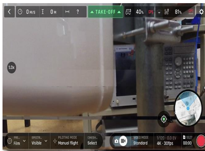
Figure 6.5: Image quality of UAV 3 for RF noise =17 dBm.
