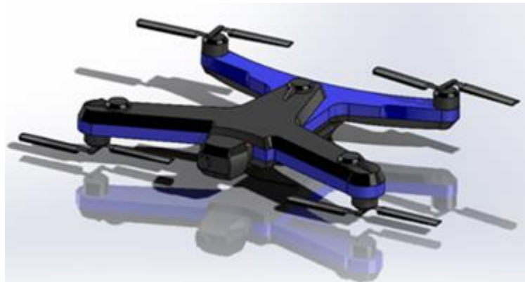
Figure 4.6: Developed Solidworks CAD model of the Skydio 2 UAV.
