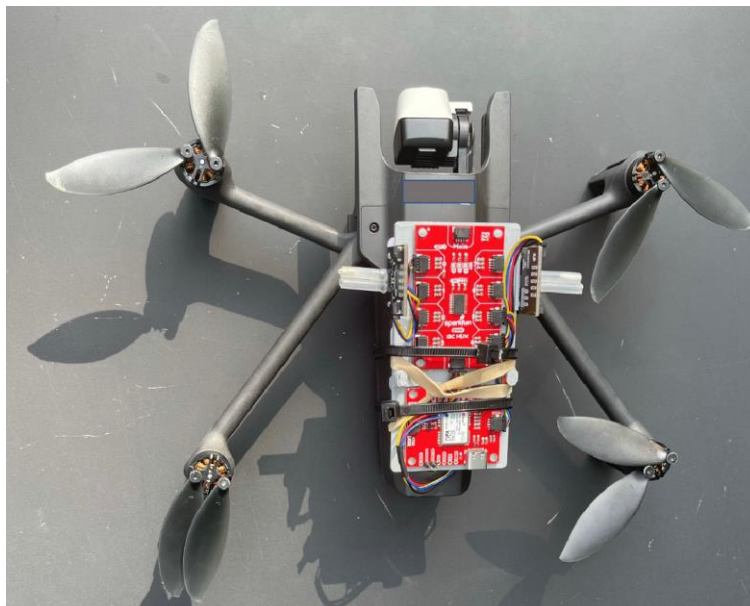
Figure 5.10: Custom flight data collection mounted on a UAV.
