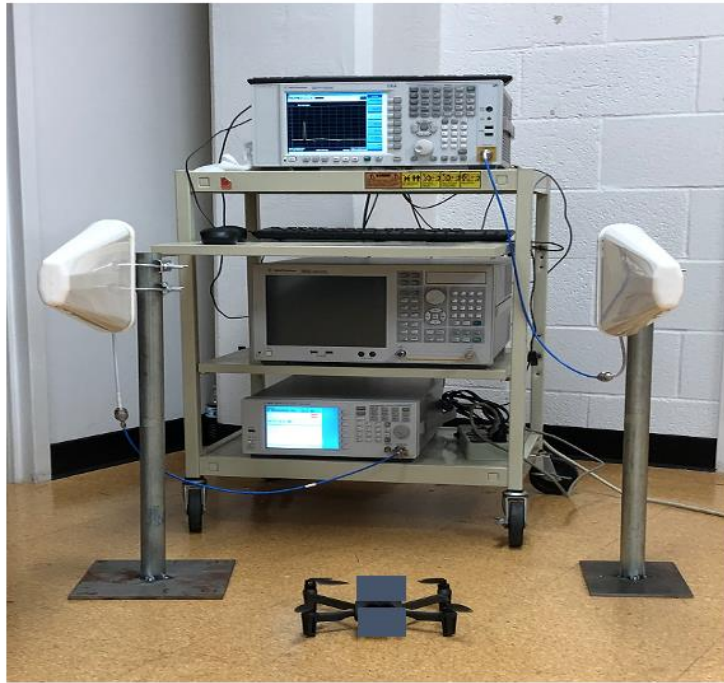
Figure 5.2: RF test setup.
