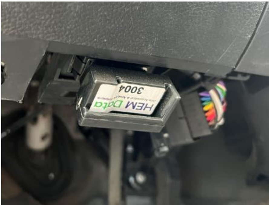
Figure 3-3. HEM Mini Logger and installation
