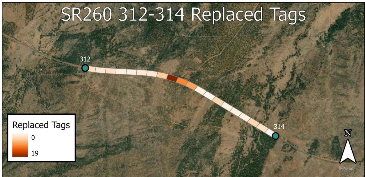
Figure 18. A heat map of replaced tag locations along SR 260 mileposts 312 to 314
