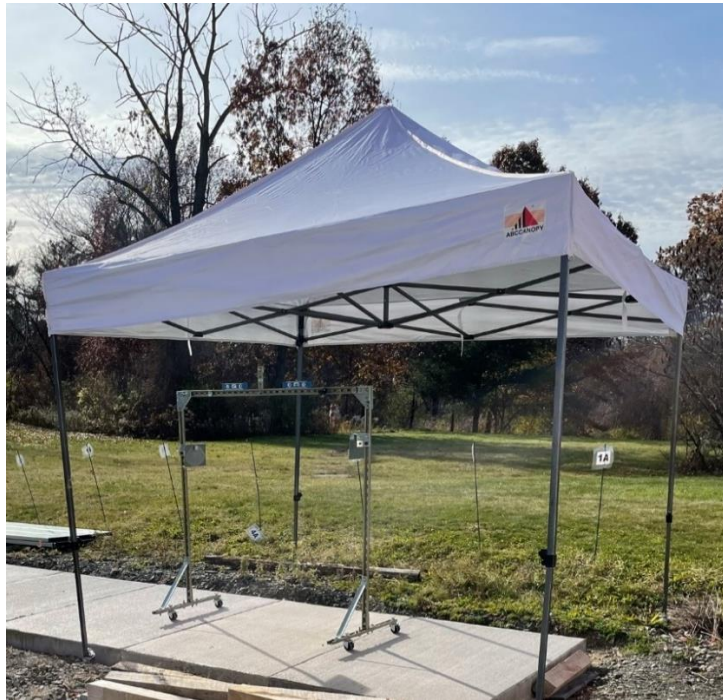
Figure 7.1 Photo rig setup to document sidewalk panels
