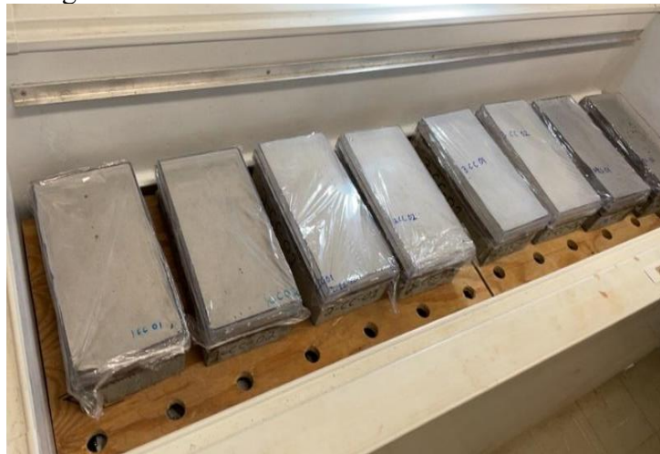
Figure 4.6 Specimens in chest freezer
