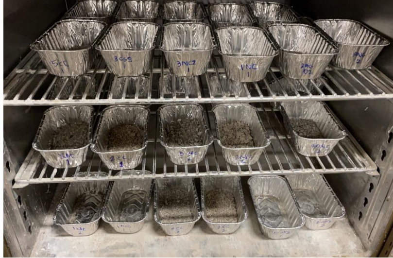
Figure 4.7 Tin foil pans containing scaled-off mass in oven for drying
