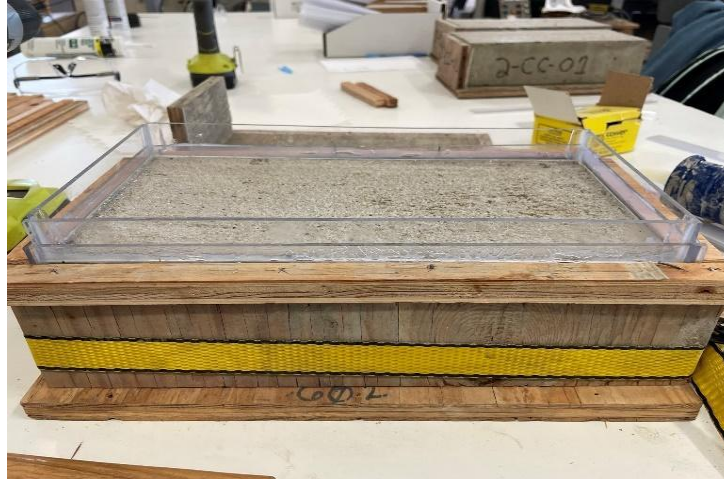
Figure 4.5 Plexiglass dikes installed on a specimen
