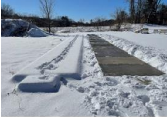
(a) Removal of snow on panels D, E, and F which are subjected to \text{MgCl}_2 (Right). Panels G, H, and I treated with blended brine on accumulated snow (Left) on February 26 th , 2022.
