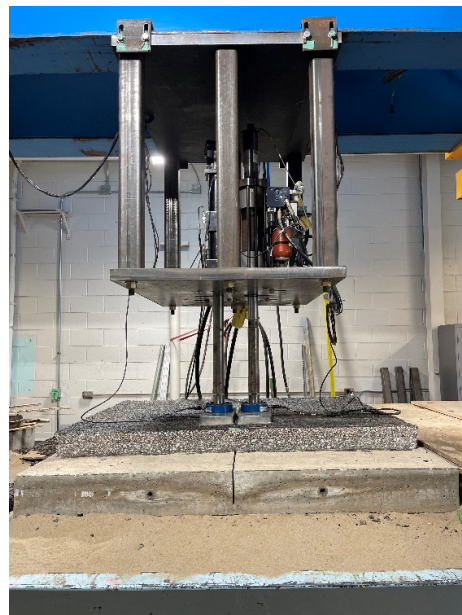
Figure 25. Photo. Hydraulic loading system.
