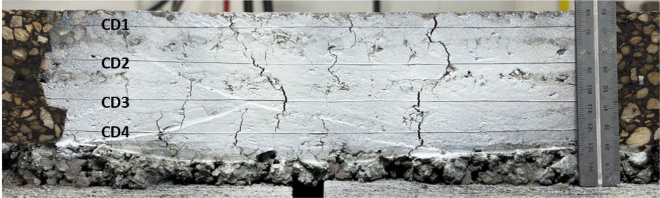
Figure 35. Photo. Interstate alternative scenario 1: cross-section after testing.
