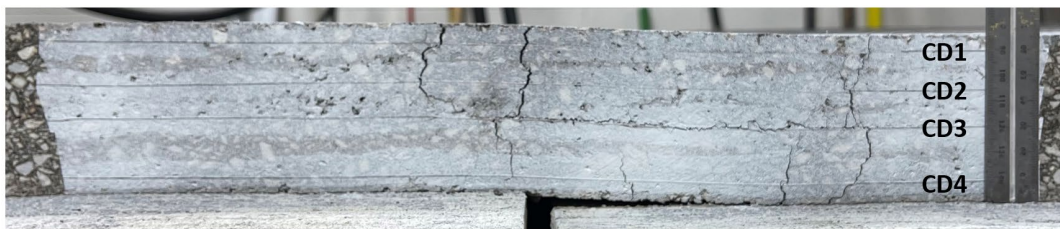
Figure 47. Photo. Non-interstate alternative scenario 1: cross-section after testing.
