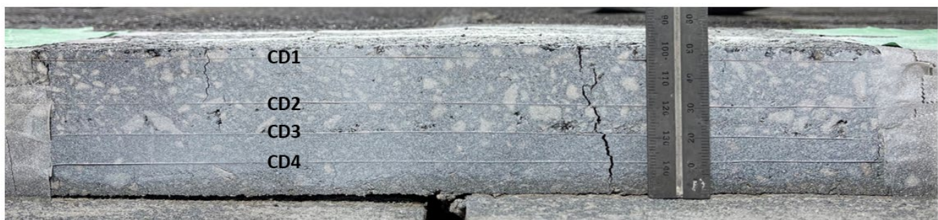
Figure 53. Photo. Non-interstate alternative scenario 3: cross-section after testing.
