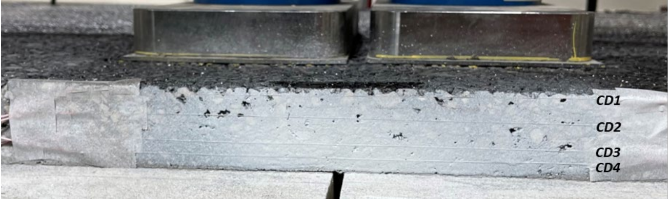
Figure 22. Photo. Copper wires glued on an HMA surface (CD1–CD4).
