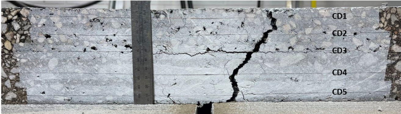
Figure 38. Photo. Interstate alternative scenario 2: cross-section after testing.
